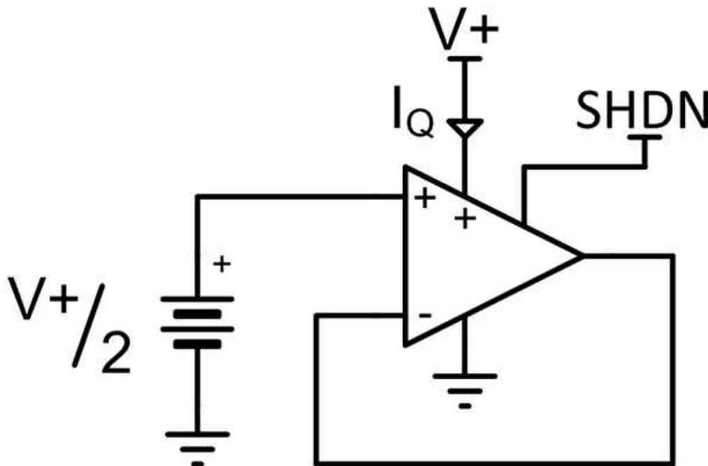
**Figure 5. TLV9042S  $I_Q$  And  $I_{QSD}$  Measurement Setup**
