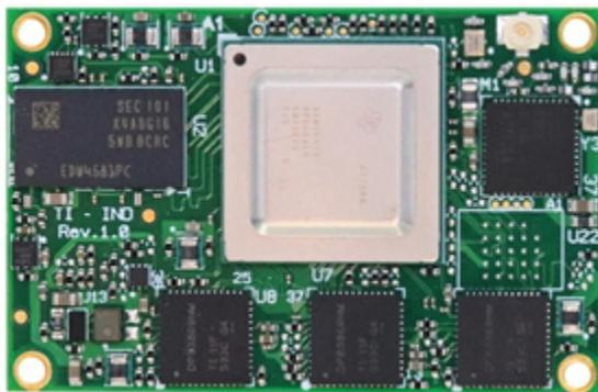
Figure 1. SolidRun's AM64x SoM Featuring AM6442. (Image Courtesy of SolidRun Ltd.)
