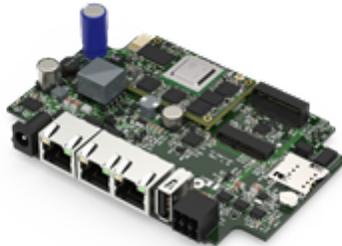
**Figure 5. SolidRun's AM64x HummingBoard-T SBC (SoM + CB) (Image Courtesy of SolidRun Ltd.)**
