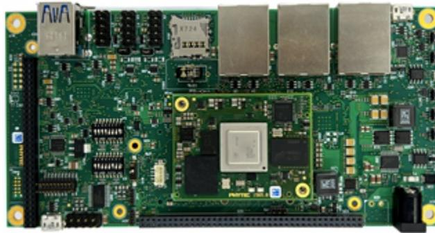
**Figure 4. Phytec's phyBOARD-AM64x-Electra Development Kit (SoM + CB). (Image Courtesy of PHYTEC)**
