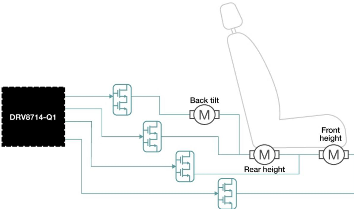
**Figure 1. A Three-motor Seat Driven by the DRV8714-Q1 Automotive Gate Driver**
