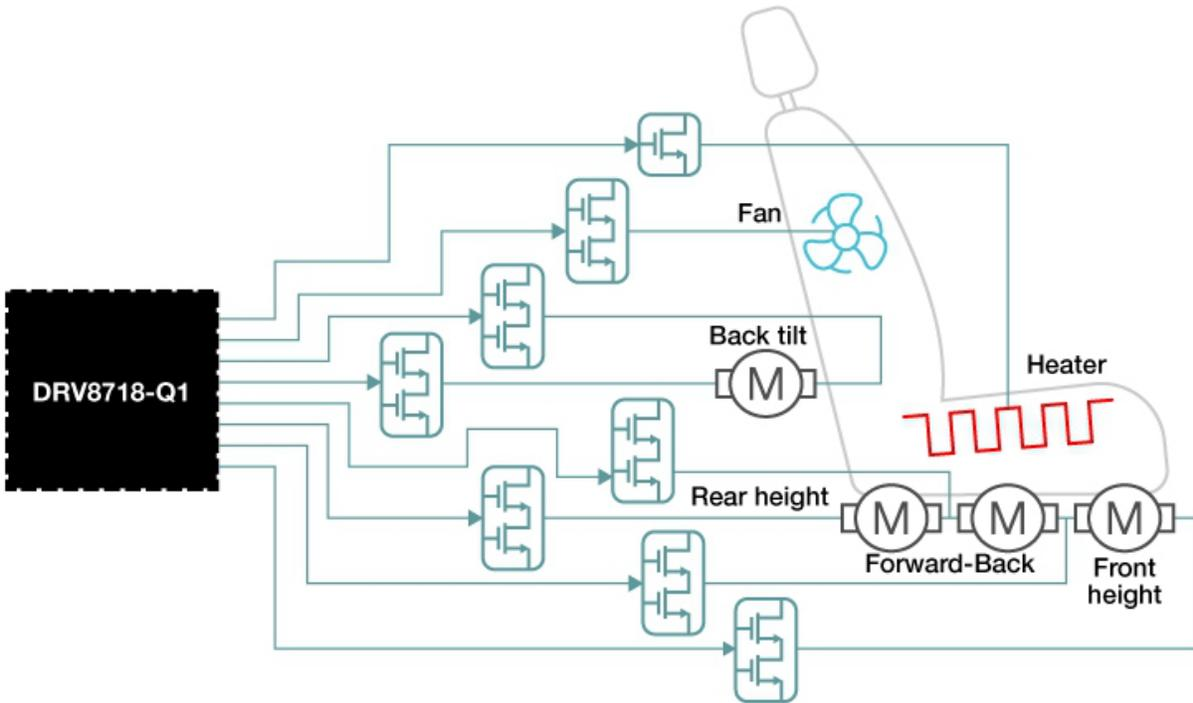
**Figure 2. The DRV8718-Q1 Automotive Gate Driver Driving Motors, a Heater and a Fan**
