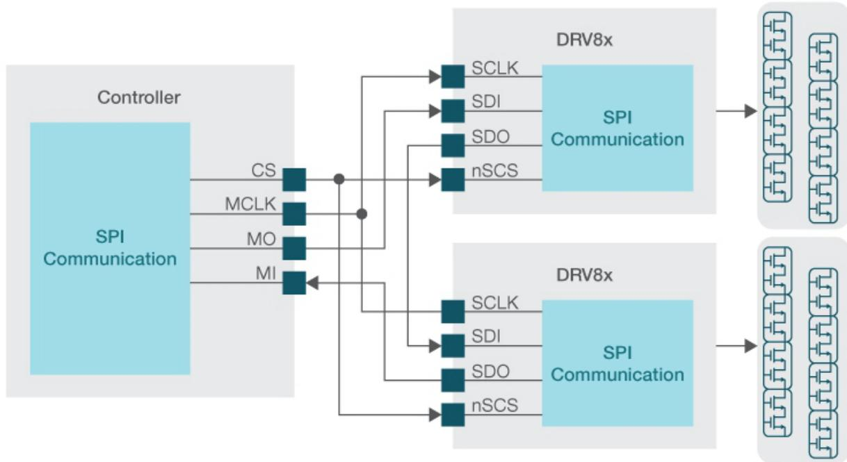
**Figure 3. Controlling 16 Half Bridges Using a Daisy-chain Configuration from the MCU to the DRV8718-Q1 Automotive Gate Driver**
