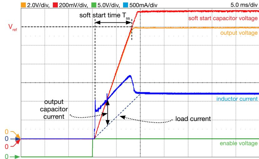
Figure 14. LM5118 Buck-Boost regulator soft start in BBM, with  $R_{17}$ ,  $C_{21}$ ,  $C_{24}$  connected (low cross-over frequency):  $V_{in}=20V$ ,  $I_{out}=1.2A$ ,  $f_s=300kHz$ ,  $R_{load}=10\Omega$ ,  $L=3.3\mu H$ ,  $C_{ss}=68nF$ .
