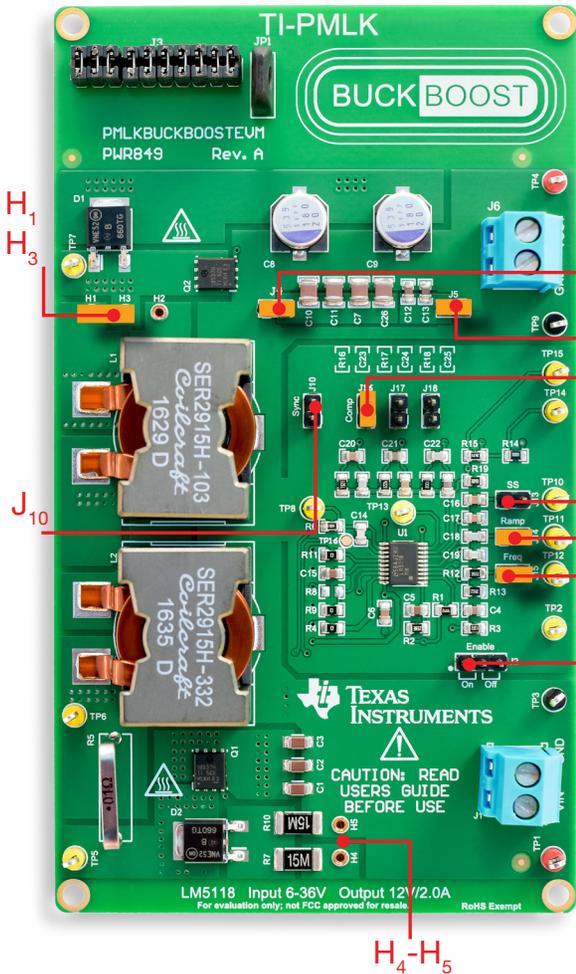
Figure 7. LM5118 board: jumpers set-up for Test#2
