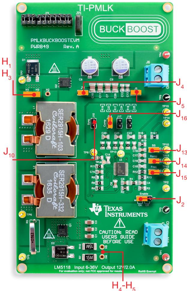
Figure 5. LM5118 board: jumpers set-up for Test#2
