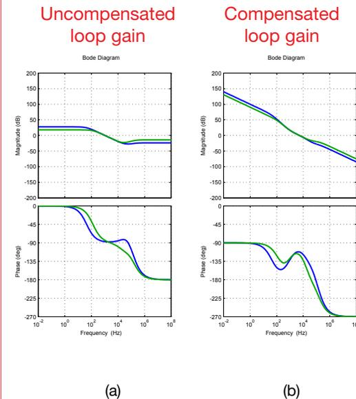
Figure 2: LM5118 loop gain in Buck-Boost Mode with inductance  $L = 10\mu\text{H}$  ( $H_1$ - $H_3$  shorted) and feedback compensation  $R_{18}$ ,  $C_{22}$ ,  $C_{25}$  connected (jumper  $J_{18}$  shorted), providing about 5kHz cross over frequency: green lines:  $V_{in}=10\text{V}@I_{out}=2\text{A}$ , blue lines:  $V_{in}=10\text{V}@I_{out}=1\text{A}$ .
