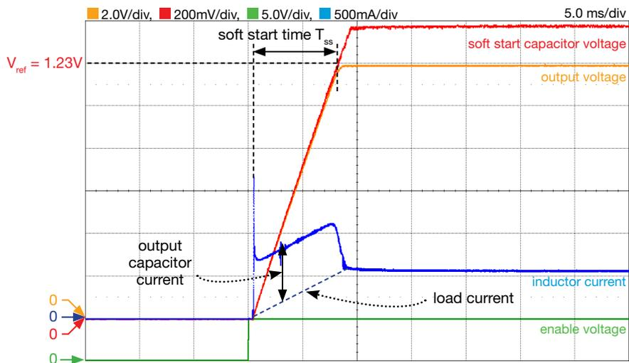
Figure 11. LM5118 Buck-Boost regulator soft start in BM, with  $R_{18}$ ,  $C_{22}$ ,  $C_{25}$  connected (high cross-over frequency):  $V_{in}=20V$ ,  $I_{out}=0.5A$ ,  $f_s=300kHz$ ,  $R_{load}=22\Omega$ ,  $L=10\mu H$ ,  $C_{ss}=68nF$ .
