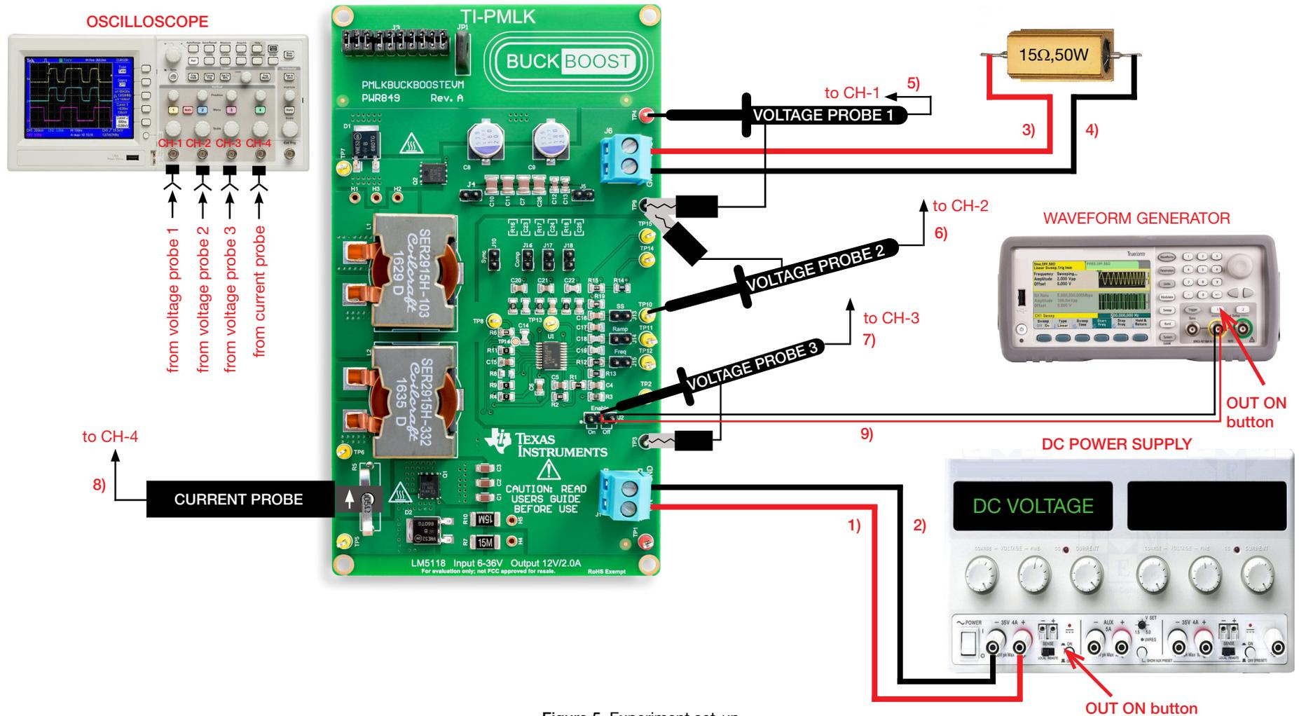
Figure 5. Experiment set-up.
