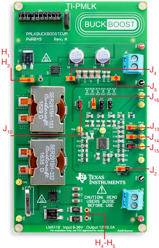
Figure 4. LM5118 board: jumpers set-up for Test#1
