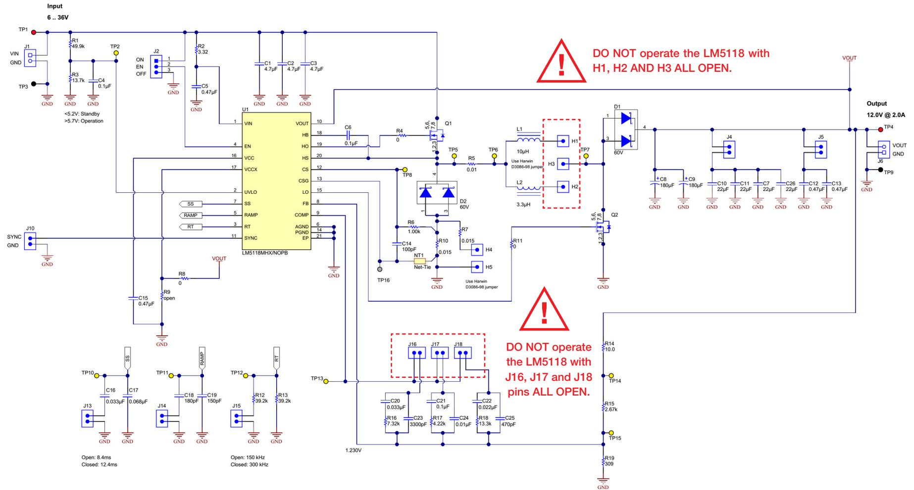
Figure 1. Circuit schematic of TI-PMLK LM5118 Buck-Boost regulator
