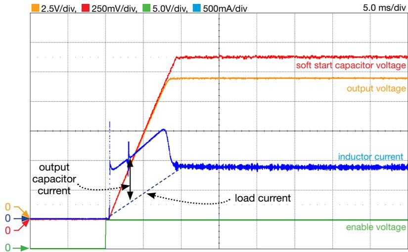
**Figure 15.** LM5118 Buck-Boost regulator soft start in BM:  $R_{18}$ ,  $C_{22}$ ,  $C_{25}$  compensation connected,  $V_{in}=20V$ ,  $I_{out}=0.8A$ ,  $f_s=300kHz$ ,  $R_{load}=15\Omega$ ,  $L=10\mu H$ ,  $C_{ss}=68nF$  and  $C_{out}=2 \times 180\mu F + 2 \times 47\mu F + 2 \times 0.47\mu F$  ( $J_{14}$  sh).
