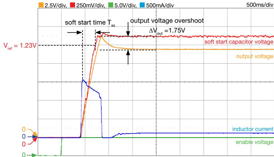
Figure 17. LM5118 Buck-Boost regulator soft start in BM, with  $R_{16}$ ,  $C_{20}$ ,  $C_{23}$  connected (low cross-over frequency):  $V_{in}=20V$ ,  $I_{out}=1.2A$ ,  $f_s=300kHz$ ,  $R_{load}=10\Omega$ ,  $L=3.3\mu H$ ,  $C_{ss}=2.2nF$ .
