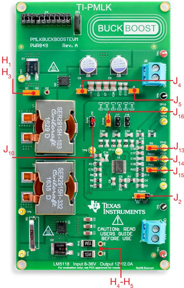
Figure 6. LM5118 board: jumpers set-up for Test#2
