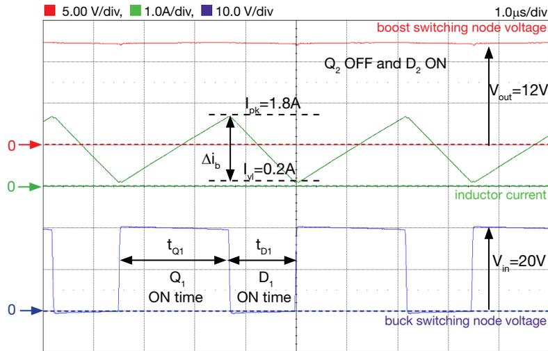
Figure 6. LM5118 regulator in steady-state CCM Buck-Boost operation:
