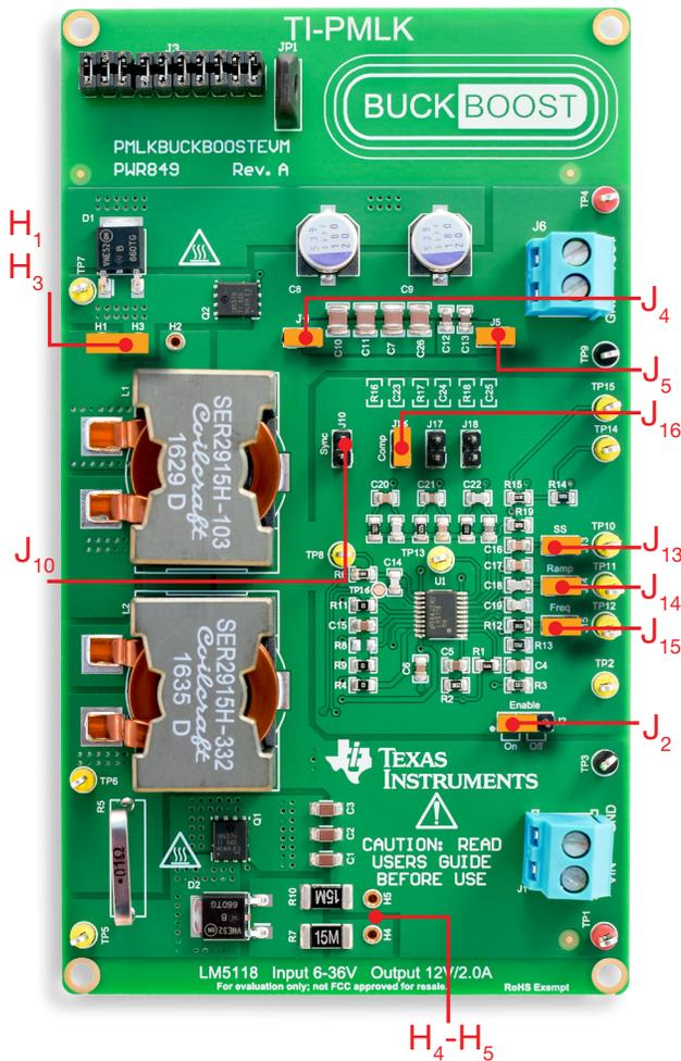
Figure 5. LM5118 board: jumpers set-up for Test#1
