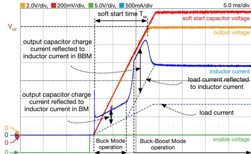
Figure 8. LM5118 Buck-Boost regulator soft start in BBM, with  $R_{18}$ ,  $C_{22}$ ,  $C_{25}$  connected (high cross-over frequency):  $V_{in}=20V$ ,  $I_{out}=0.8A$ ,  $f_s=300kHz$ ,  $R_{load}=15\Omega$ ,  $L=10\mu H$ ,  $C_{ss}=110nF$ .
