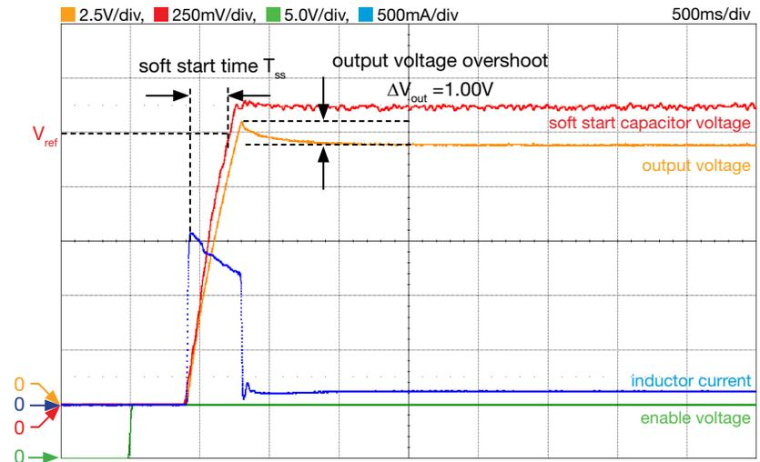
Figure 18. LM5118 Buck-Boost regulator soft start in BBM, with  $R_{18}$ ,  $C_{22}$ ,  $C_{25}$  connected (high cross-over frequency):  $V_{in}=20V$ ,  $I_{out}=1.2A$ ,  $f_s=300kHz$ ,  $R_{load}=10\Omega$ ,  $L=3.3\mu H$ ,  $C_{ss}=2.2nF$ .
