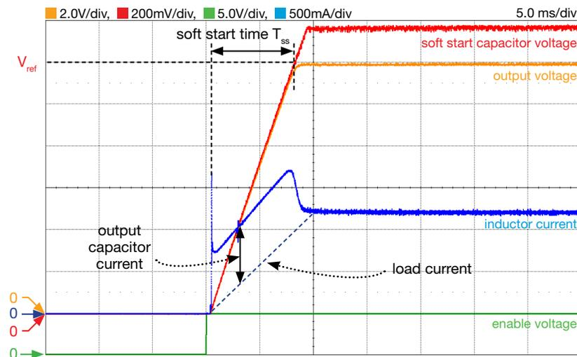
Figure 12. LM5118 Buck-Boost regulator soft start in BBM, with  $R_{18}$ ,  $C_{22}$ ,  $C_{25}$  connected (high cross-over frequency):  $V_{in}=20V$ ,  $I_{out}=1.2A$ ,  $f_s=300kHz$ ,  $R_{load}=10\Omega$ ,  $L=10\mu H$ ,  $C_{ss}=68nF$ .
