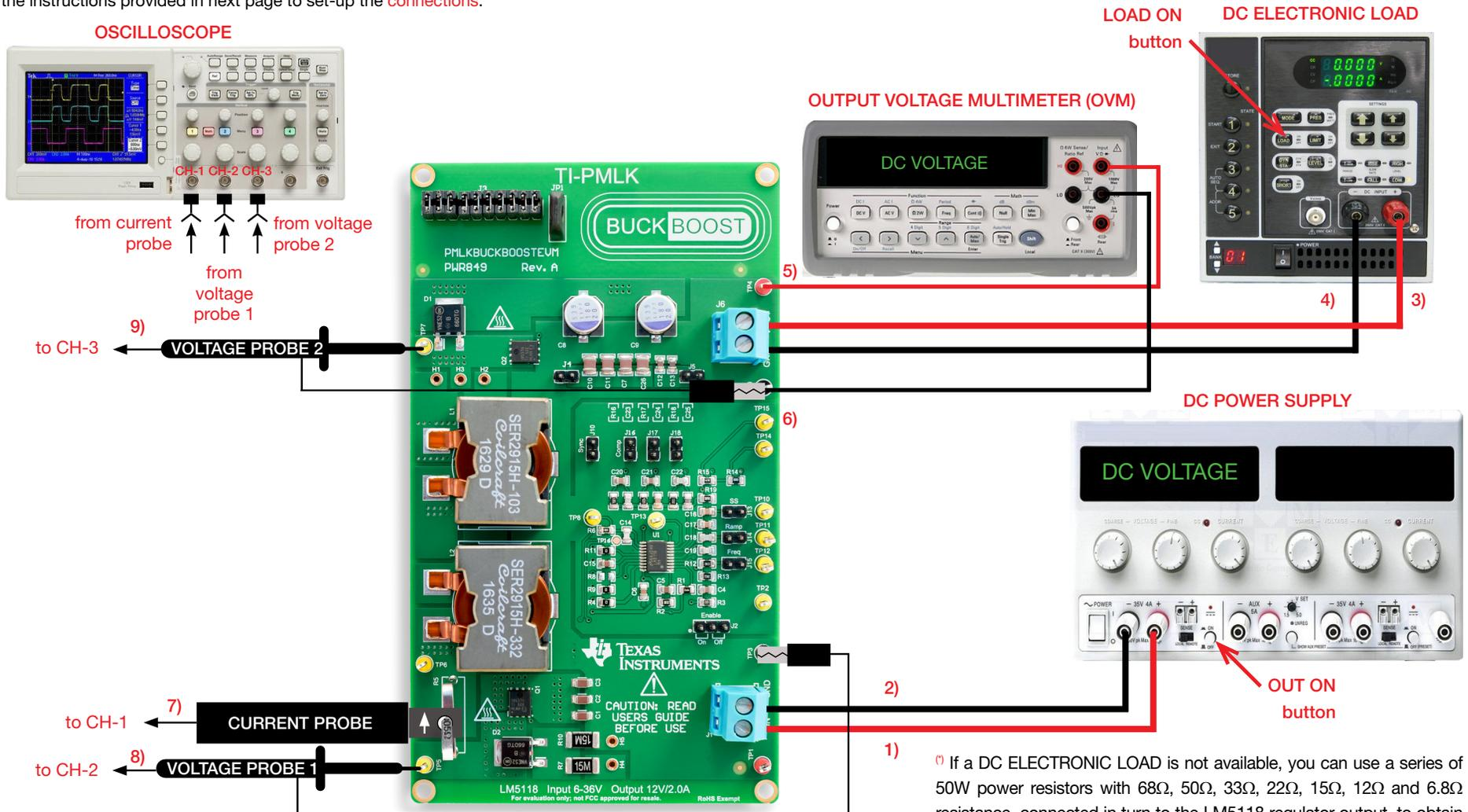
Figure 3. Experiment set-up.
