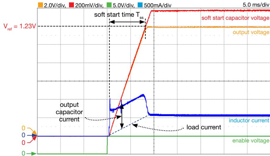
Figure 13. LM5118 Buck-Boost regulator soft start in BM, with  $R_{17}$ ,  $C_{21}$ ,  $C_{24}$  connected (low cross-over frequency):  $V_{in}=20V$ ,  $I_{out}=0.5A$ ,  $f_s=300kHz$ ,  $R_{load}=22\Omega$ ,  $L=3.3\mu H$ ,  $C_{ss}=68nF$ .
