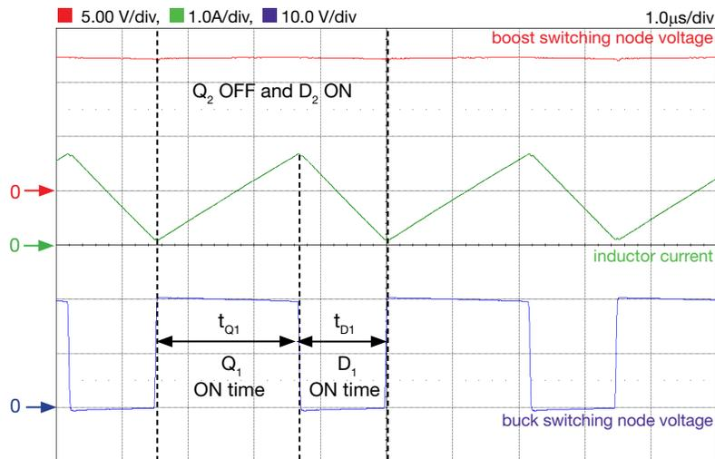
Figure 8. LM5118 regulator in steady-state CCM Buck-Boost operation:
