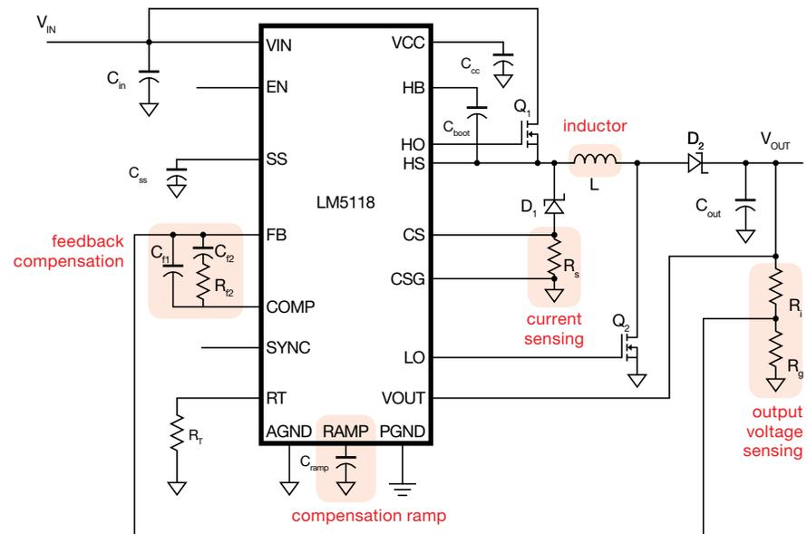
Figure 1. Simplified schematic of the LM5118 Buck-Boost regulator
