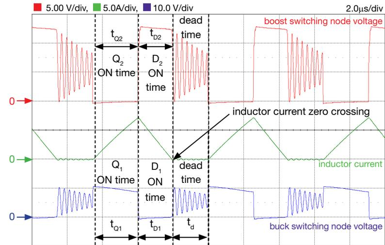
Figure 11. LM5118 regulator in steady-state DCM Buck-Boost operation:
