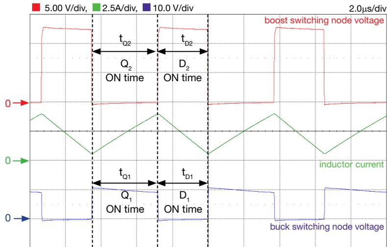
Figure 10. LM5118 regulator in steady-state CCM Buck-Boost operation:
