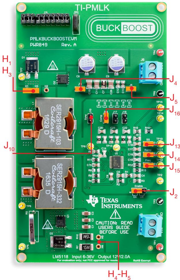
Figure 6. LM5118 board: jumpers set-up for Test#1
