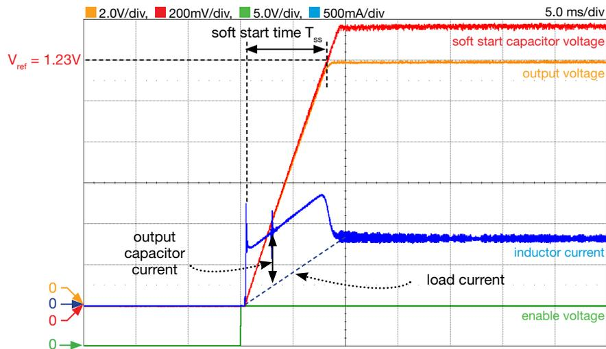
Figure 9. LM5118 Buck-Boost regulator soft start in BM, with  $R_{16}$ ,  $C_{20}$ ,  $C_{23}$  connected (low cross-over frequency):  $V_{in}=20V$ ,  $I_{out}=0.8A$ ,  $f_s=300kHz$ ,  $R_{load}=15\Omega$ ,  $L=10\mu H$ ,  $C_{ss}=68nF$ .
