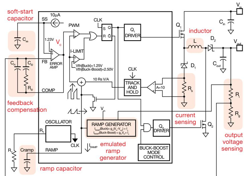
Figure 1. Simplified schematic of the LM5118 Buck-Boost regulator
