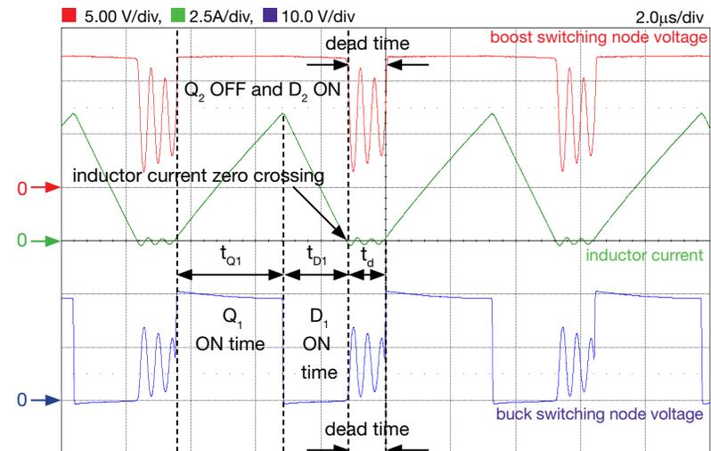
Figure 9. LM5118 regulator in steady-state DCM Buck operation:
