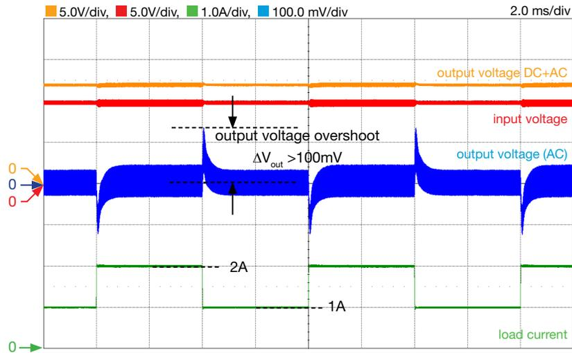
Figure 7. LM5118 buck-boost regulator load transient response in BBM, with  $R_{16}$ ,  $C_{20}$ ,  $C_{23}$  connected (lower cross-over frequency):  $V_{in}=10V$ ,  $I_{out}=1.0A$  to  $2.0A$ ,  $f_s=300kHz$ ,  $L=10\mu H$
