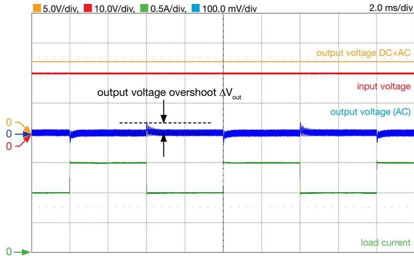
Figure 13. LM5118 Buck-Boost regulator load transient response in BM, with  $R_{16}$ ,  $C_{20}$ ,  $C_{23}$  connected (low cross-over frequency):  $V_{in}=20V$ ,  $I_{out}=1.0A$  to  $1.5A$ ,  $f_s=300kHz$ ,  $L=10\mu H$
