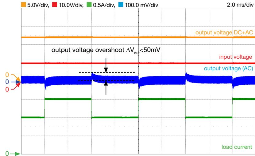
Figure 12. LM5118 Buck-Boost regulator load transient response in BBM, with  $R_{17}$ ,  $C_{21}$ ,  $C_{24}$  connected (low cross-over frequency):  $V_{in}=10V$ ,  $I_{out}=1.0A$  to  $1.5A$ ,  $f_s=300kHz$ ,  $L=3.3\mu H$
