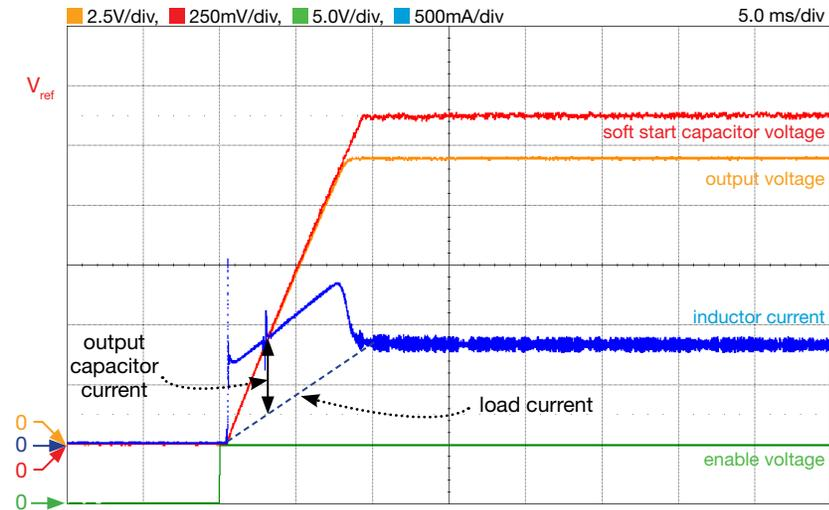
**Figure 16.** LM5118 Buck-Boost regulator soft start in BM:  $R_{18}$ ,  $C_{22}$ ,  $C_{25}$  compensation connected,  $V_{in}=20V$ ,  $I_{out}=0.8A$ ,  $f_s=300kHz$ ,  $R_{load}=15\Omega$ ,  $L=10\mu H$ ,  $C_{ss}=68nF$  and  $C_{out}=2 \times 180\mu F + 2 \times 0.47\mu F$  ( $J_{14}$  op).
