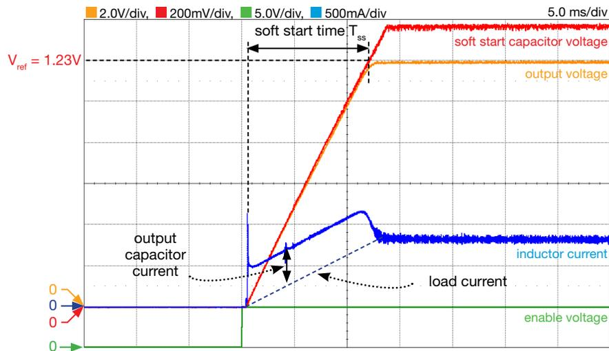
Figure 7. LM5118 Buck-Boost regulator soft start in BM, with  $R_{18}$ ,  $C_{22}$ ,  $C_{25}$  connected (high cross-over frequency):  $V_{in}=20V$ ,  $I_{out}=0.8A$ ,  $f_s=300kHz$ ,  $R_{load}=15\Omega$ ,  $L=10\mu H$ ,  $C_{ss}=110nF$ .
