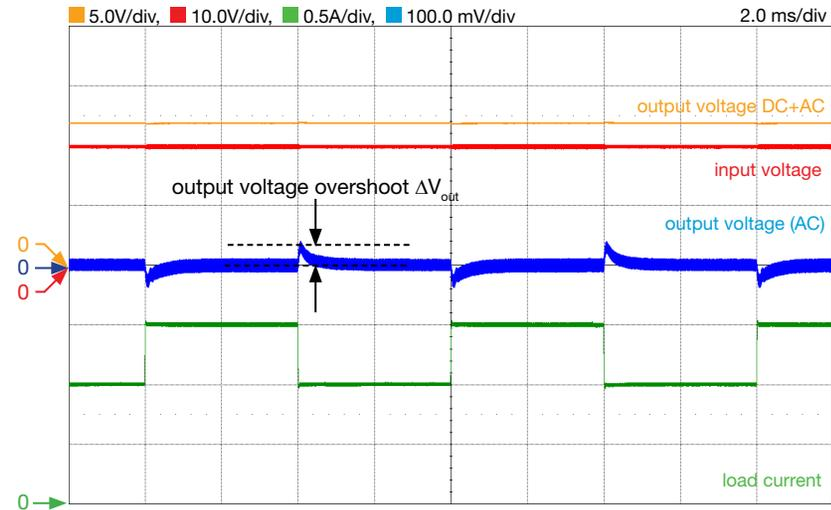
Figure 14. LM5118 Buck-Boost regulator load transient response in BM, with  $R_{17}$ ,  $C_{21}$ ,  $C_{24}$  connected (low cross-over frequency):  $V_{in}=20V$ ,  $I_{out}=1.0A$  to  $1.5A$ ,  $f_s=300kHz$ ,  $L=3.3\mu H$
