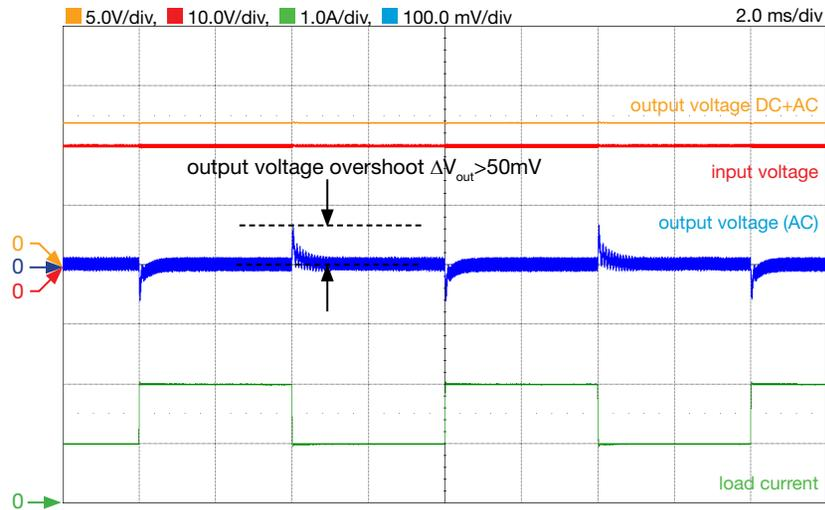
Figure 9. LM5118 Buck-Boost regulator load transient response in BM, with  $R_{18}$ ,  $C_{20}$ ,  $C_{23}$  connected (lower cross-over frequency):  $V_{in}=20\text{V}$ ,  $I_{out}=1.0\text{A}$  to  $2.0\text{A}$ ,  $f_s=300\text{kHz}$ ,  $L=10\mu\text{H}$
