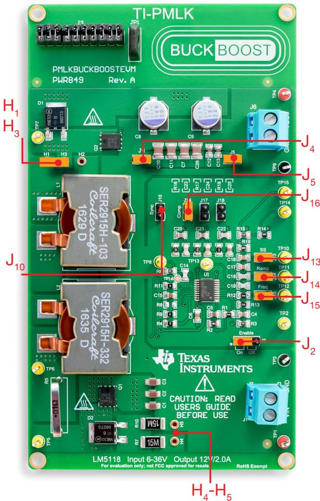
Figure 7. LM5118 board: jumpers set-up for Test#2
