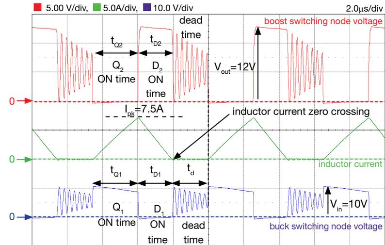
Figure 9. LM5118 regulator in steady-state DCM Buck-Boost operation:
