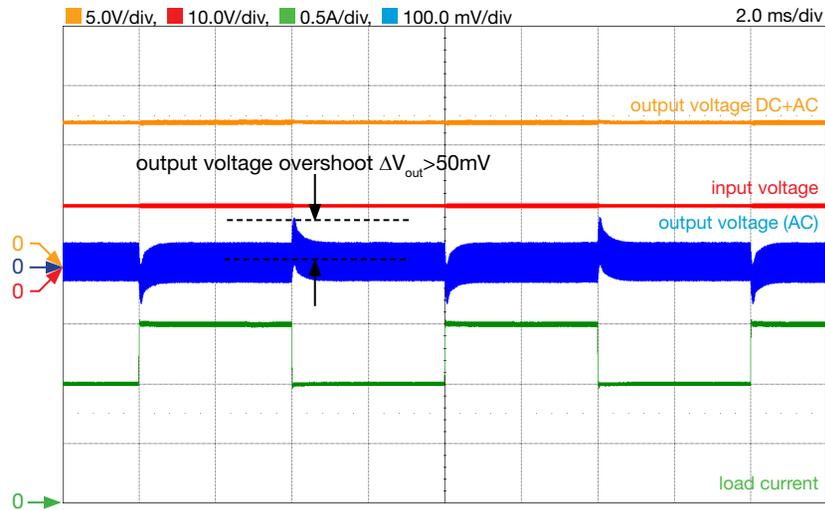
Figure 11. LM5118 Buck-Boost regulator load transient response in BBM, with  $R_{16}$ ,  $C_{20}$ ,  $C_{23}$  connected (low cross-over frequency):  $V_{in}=10V$ ,  $I_{out}=1.0A$  to  $1.5A$ ,  $f_s=300kHz$ ,  $L=10\mu H$
