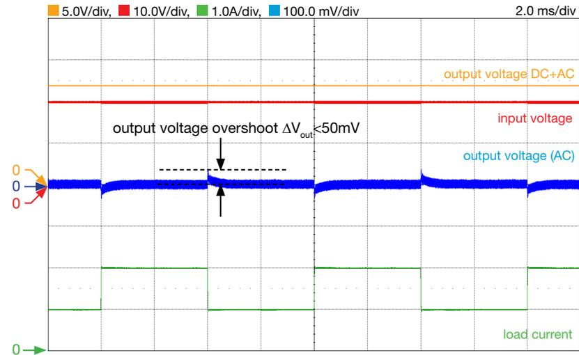
Figure 10. LM5118 Buck-Boost regulator load transient response in BM, with  $R_{18}$ ,  $C_{22}$ ,  $C_{25}$  connected (higher cross-over frequency):  $V_{in}=20\text{V}$ ,  $I_{out}=1.0\text{A}$  to  $2.0\text{A}$ ,  $f_s=300\text{kHz}$ ,  $L=10\mu\text{H}$
