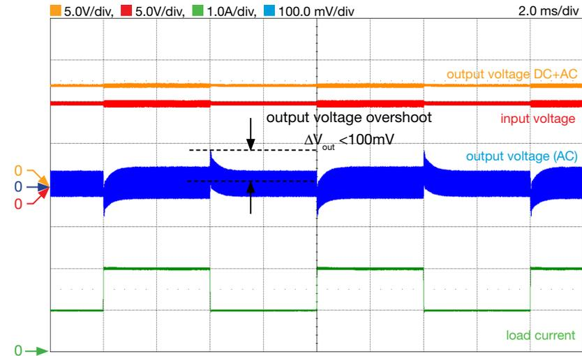
Figure 8. LM5118 buck-boost regulator load transient response in BBM, with  $R_{18}$ ,  $C_{22}$ ,  $C_{25}$  connected (higher cross-over frequency):  $V_{in}=10V$ ,  $I_{out}=1.0A$  to  $2.0A$ ,  $f_s=300kHz$ ,  $L=10\mu H$
