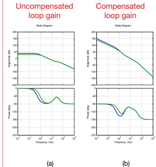
Figure 3: LM5118 loop gain in Buck Mode with inductance  $L = 10\mu\text{H}$  ( $H_1$ - $H_3$  shorted) and feedback compensation  $R_{18}$ ,  $C_{22}$ ,  $C_{25}$  connected (jumper  $J_{18}$  shorted), providing about 10kHz cross over frequency: green lines:  $V_{in}=20\text{V}@I_{out}=2\text{A}$ , blue lines:  $V_{in}=20\text{V}@I_{out}=1\text{A}$ .
