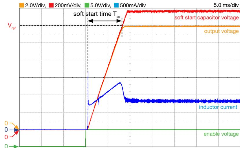
Figure 10. LM5118 Buck-Boost regulator soft start in BBM, with  $R_{18}$ ,  $C_{22}$ ,  $C_{25}$  connected (high cross-over frequency):  $V_{in}=20V$ ,  $I_{out}=0.8A$ ,  $f_s=300kHz$ ,  $R_{load}=15\Omega$ ,  $L=10\mu H$ ,  $C_{ss}=68nF$ .
