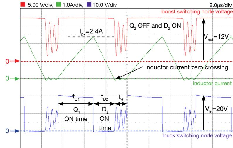
Figure 7. LM5118 regulator in steady-state CCM Buck operation:
