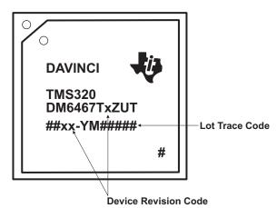
Figure 1. Example, Device Revision Codes for TMS320DM6467T (ZUT Package)
