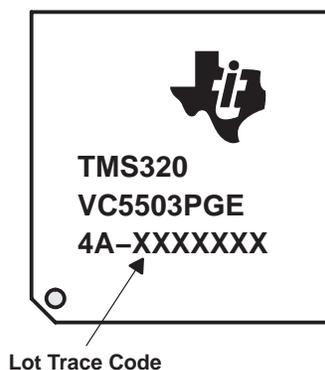
Figure 1. Example Markings for VC5503, PGE Package, Revision 1.0
