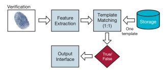
Figure 3: Biometrics verification process
