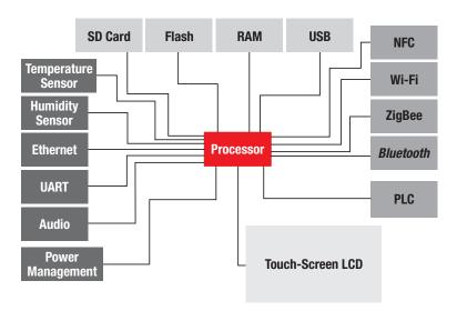
Figure 1. Smart thermostat architecture
