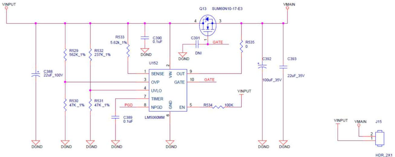
Figure 20. Overvoltage Fault Indicator
