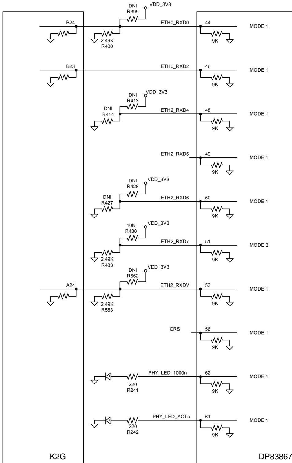
Consult the data manual of the DP83867 for more details on configuring the PHY. The DP83867 strapping can be read from the STRAP\_STS1 and STRAP\_STS2 registers. The strapping resistors on the K2G ICE configures the DP83867, as show in [Table 3](#).
