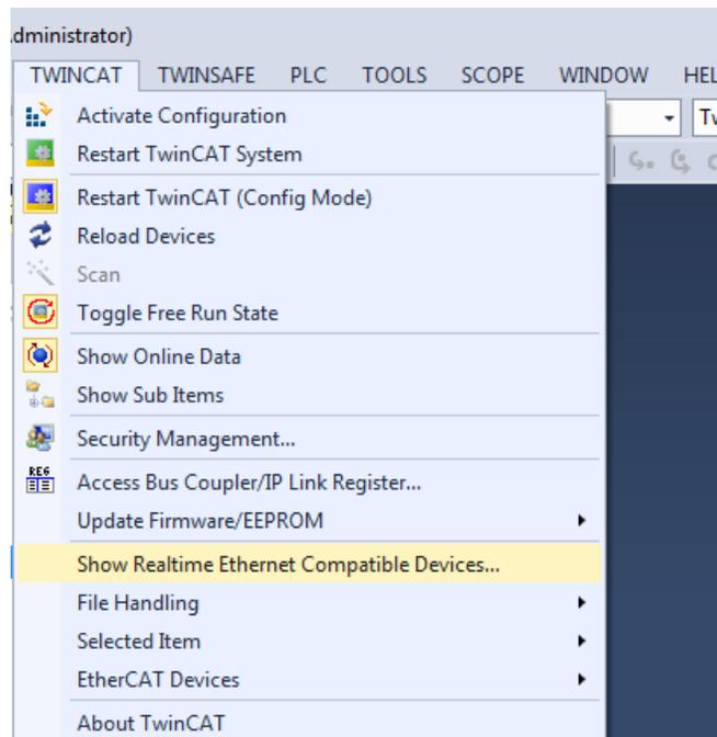
5. Select the Ethernet port from the list of compatible devices, and press Install. This installs a Beckhoff EtherCAT driver. When installed, the Ethernet port appears in Installed and ready to use devices, as shown in [Figure 10](#).
