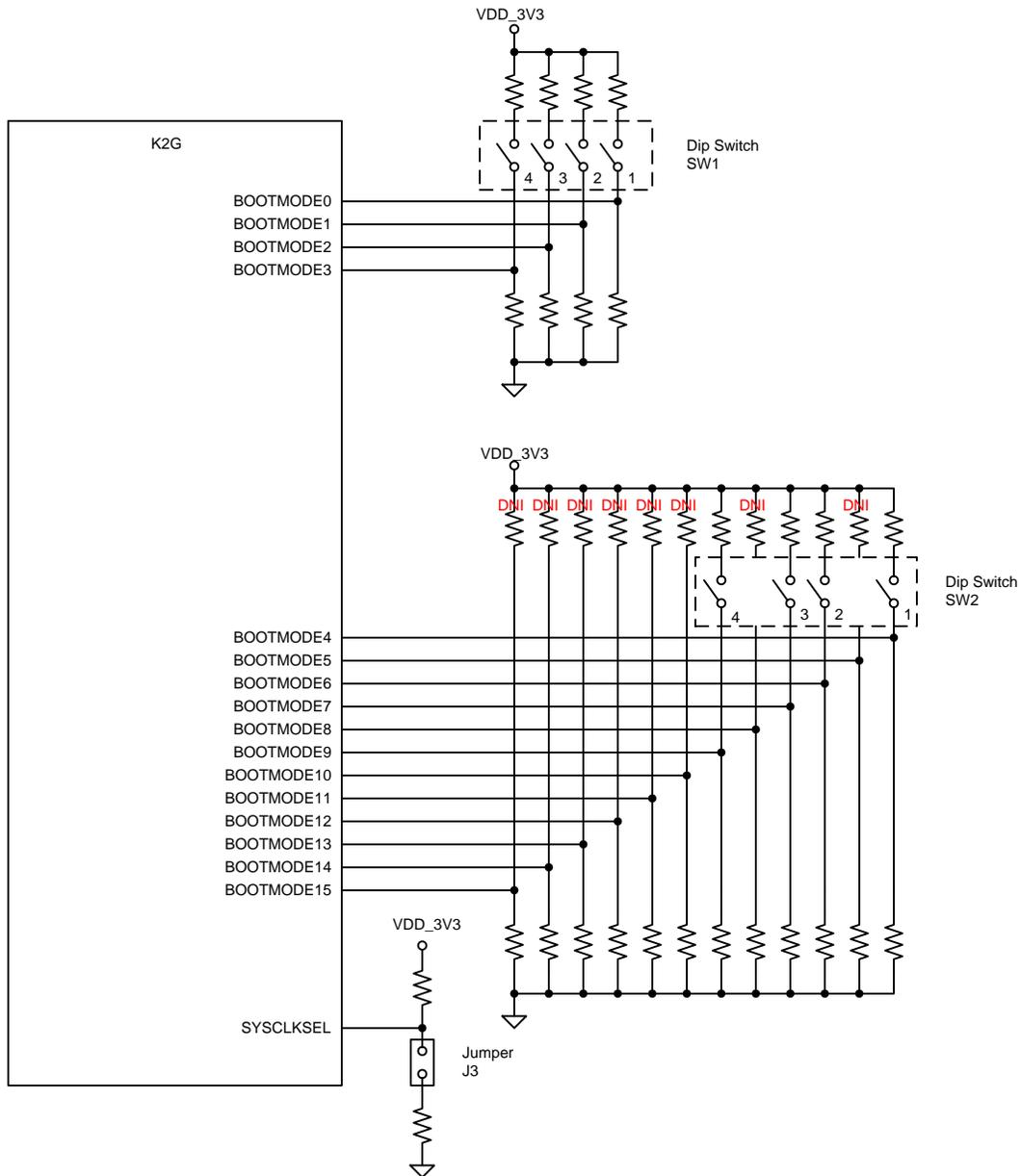
The dip switches are located just above the expansion connector, as shown in [Figure 24](#). Bootmode switches should be set before any expansion board is installed.
