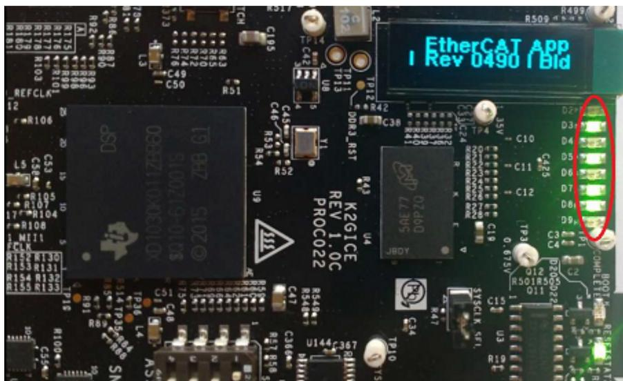
The K2G ICE is now acting as an EtherCAT slave, and the industrial LEDs can be lit using instructions from an EtherCAT master using the TwinCAT application. Instructions for installing and operating the TwinCAT application can be found in the K2G ICE User's Guide.
