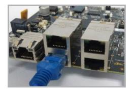
Connect the Ethernet cable between K2G ICE EtherCAT IN/
