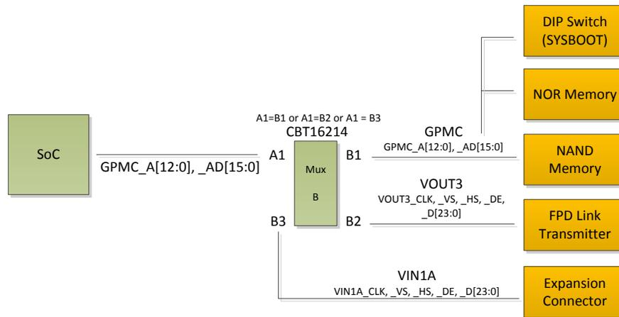
Figure 10. Mux Diagram for GPMC/VIN1/VOUT3
