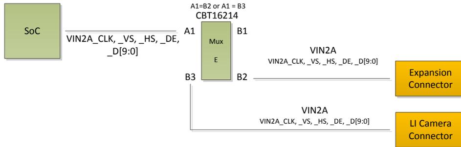
Figure 14. Mux Diagram for VIN2A and EMU
