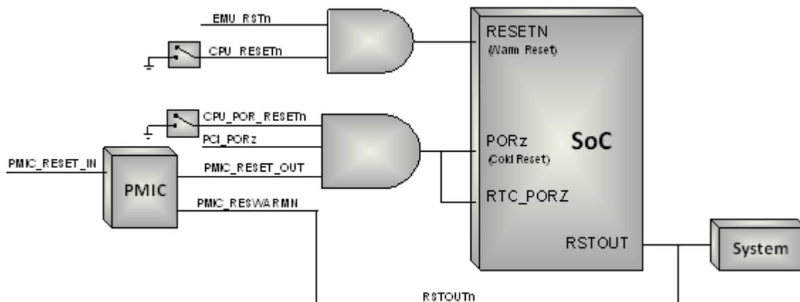
**Figure 6. Reset Structure**
