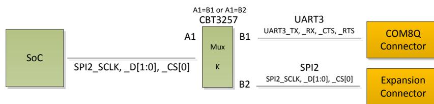
Figure 20. Mux Diagram for SPI2 and UART3
