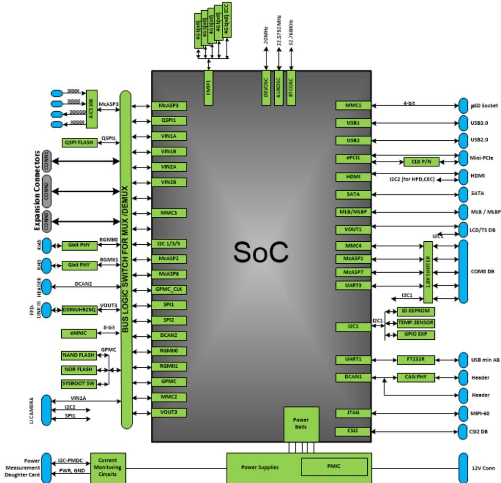
Figure 4. CPU Board Block Diagram
