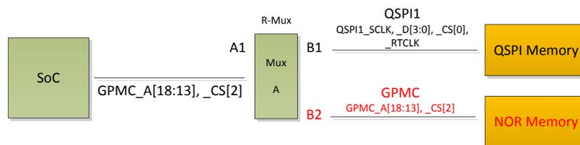
Figure 8. Mux Diagram for GPMC and QSPI
