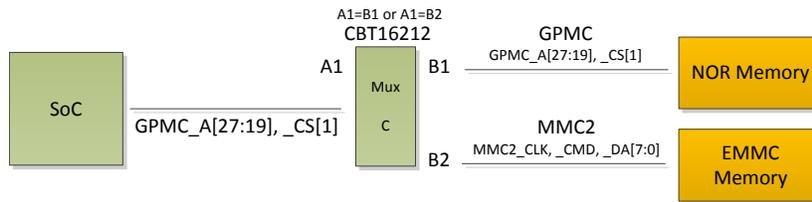
Figure 12. Mux Diagram for GPMC and EMMC
