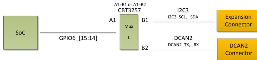
Figure 22. Mux Diagram for DCAN2 and I2C
