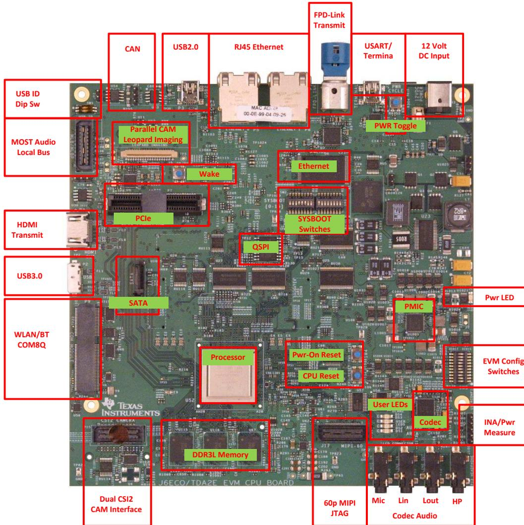
Figure 2. CPU Board – Front
