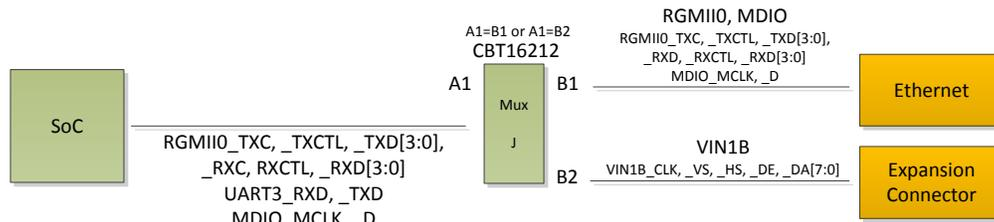
Figure 18. Mux Diagram for RGMII0 and VIN1B
