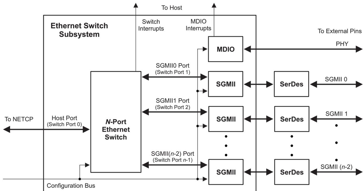
The SGMII modules connect through a SerDes to external pins, and have the Ethernet switch as their source. All SGMII modules in the subsystem follow the same protocol and methods.
