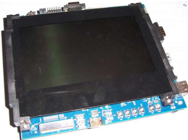
Figure 1. AM437x GP EVM Top View
