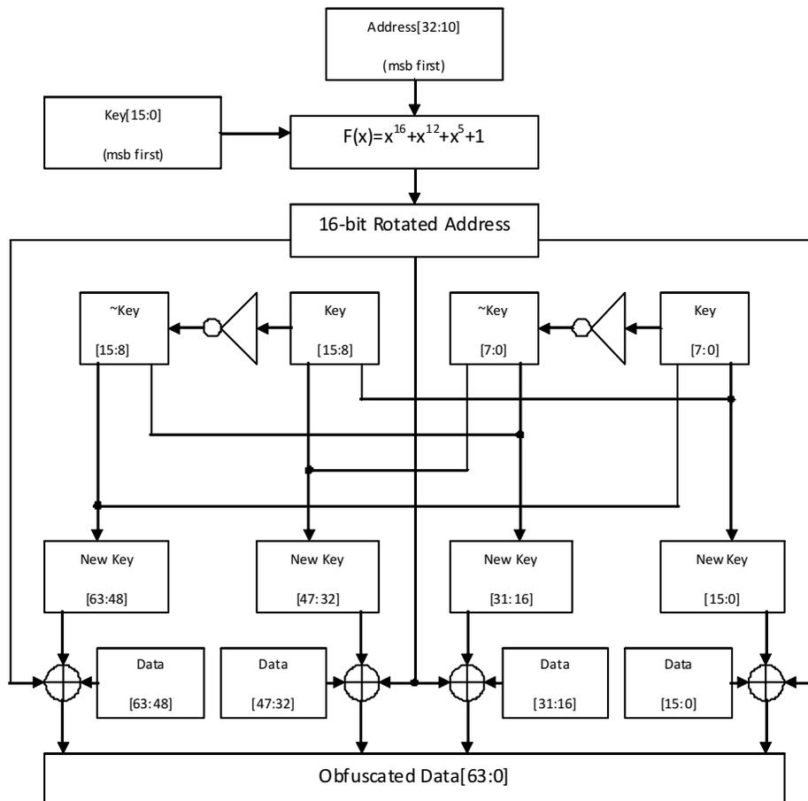
Obfuscation is enabled by setting the **OBFUSCATION\_ENABLE** bit inside the Security Manager to 1. This causes the obfuscation key to be latched inside the controller. The 16-bit key should be programmed by software inside the Security Manager.
