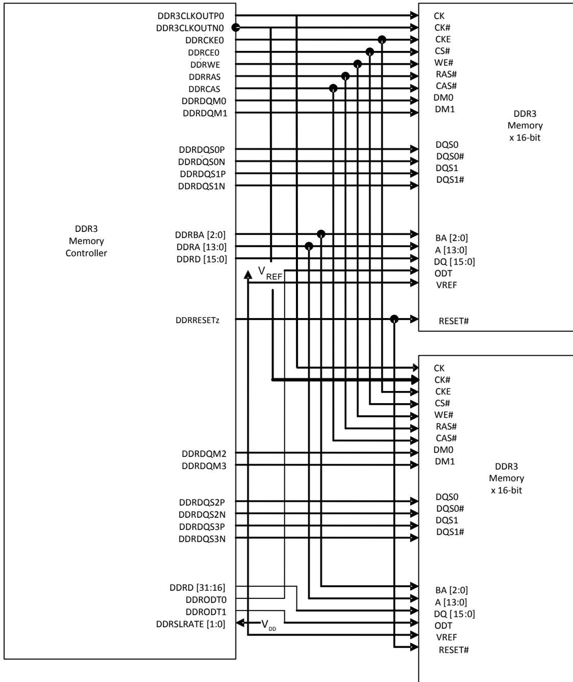
Figure 3-2. Connecting One 8 MB x 16 x 8 Banks (1Gb Total) Device
