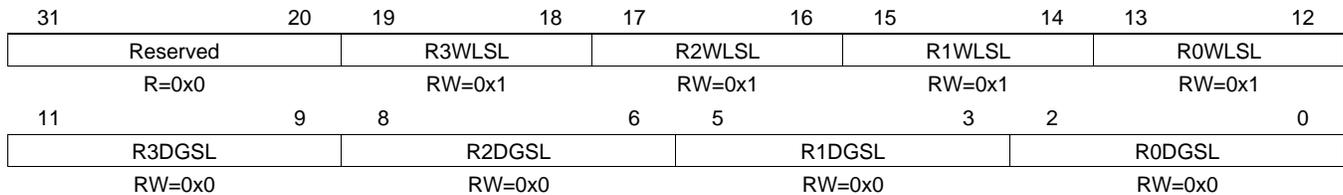
Legend: R = Read only; W = Write only; - n = value after reset; -x, value is indeterminate — see the device-specific data manual
