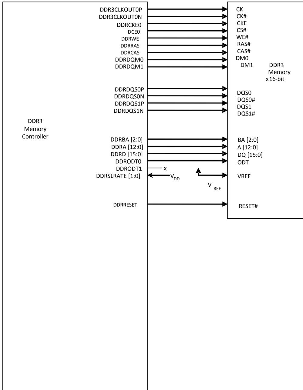
Figure 3-3. Connecting Two 16 MB x 8 x 8 Banks (2Gb Total) Devices
