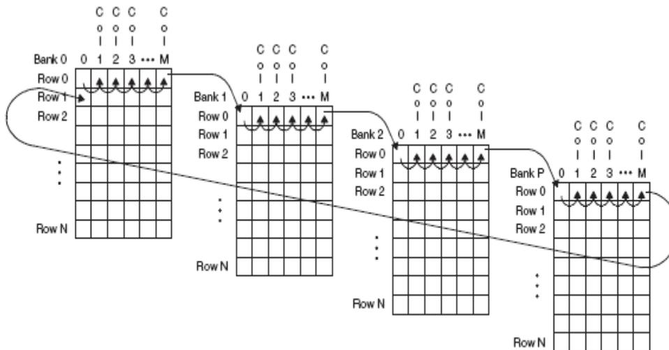
A M is number of columns (as determined by PAGESIZE) minus 1, P is number of banks (as determined by IBANK) minus 1, and N is number of rows (as determined by both PAGESIZE and IBANK) minus 1.
