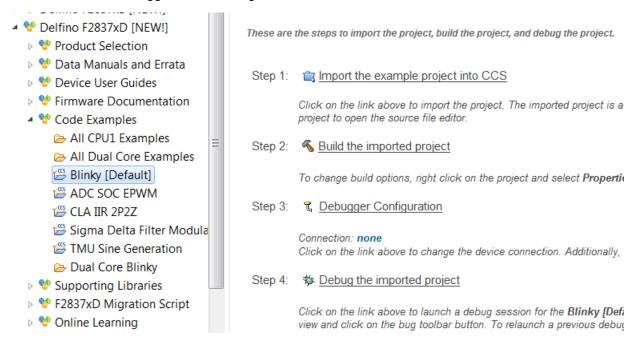
Figure 9. Example of Project Importing through the GUI
