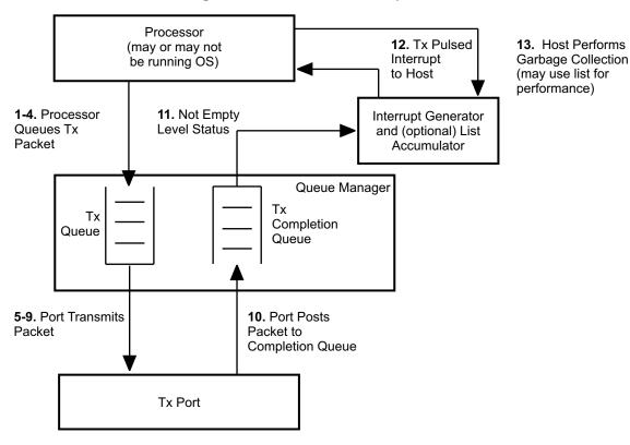
Figure 2-2. Packet Transmit Operation
