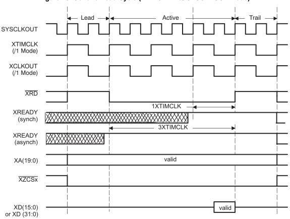
Figure 13. Generic Read Cycle (XTIMCLK = 1/2 SYSCLKOUT mode)
