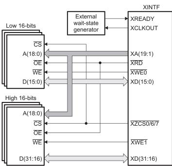
Figure 5. Typical 32-bit Data Bus XINTF Connections
