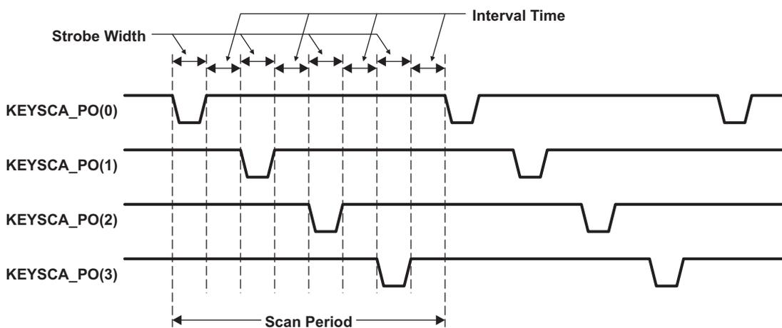
Figure 7. Channel Interval Mode at 5x3
