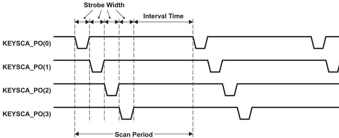
**Figure 5. Scan Interval Mode at 5x3**
