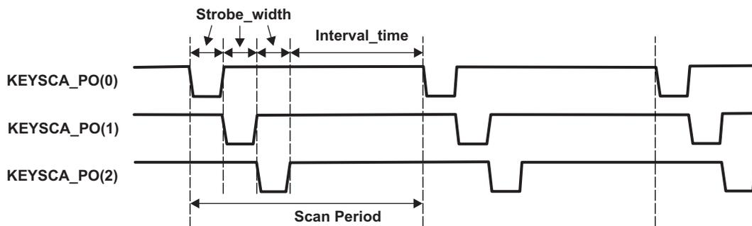
**Figure 6. Channel Interval at 4x4 Mode**
