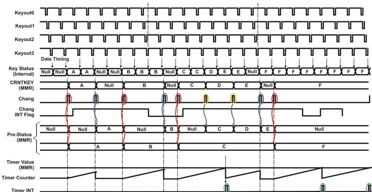
Red shows the interrupt generated when the UPDATE method is in first-switch mode.
