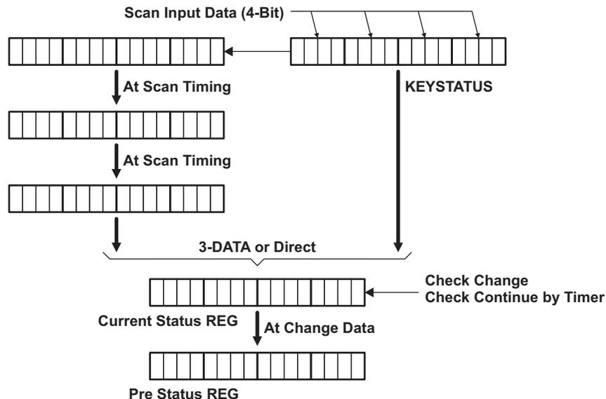
**Figure 11. Auto Detect Mode at 4x4**
