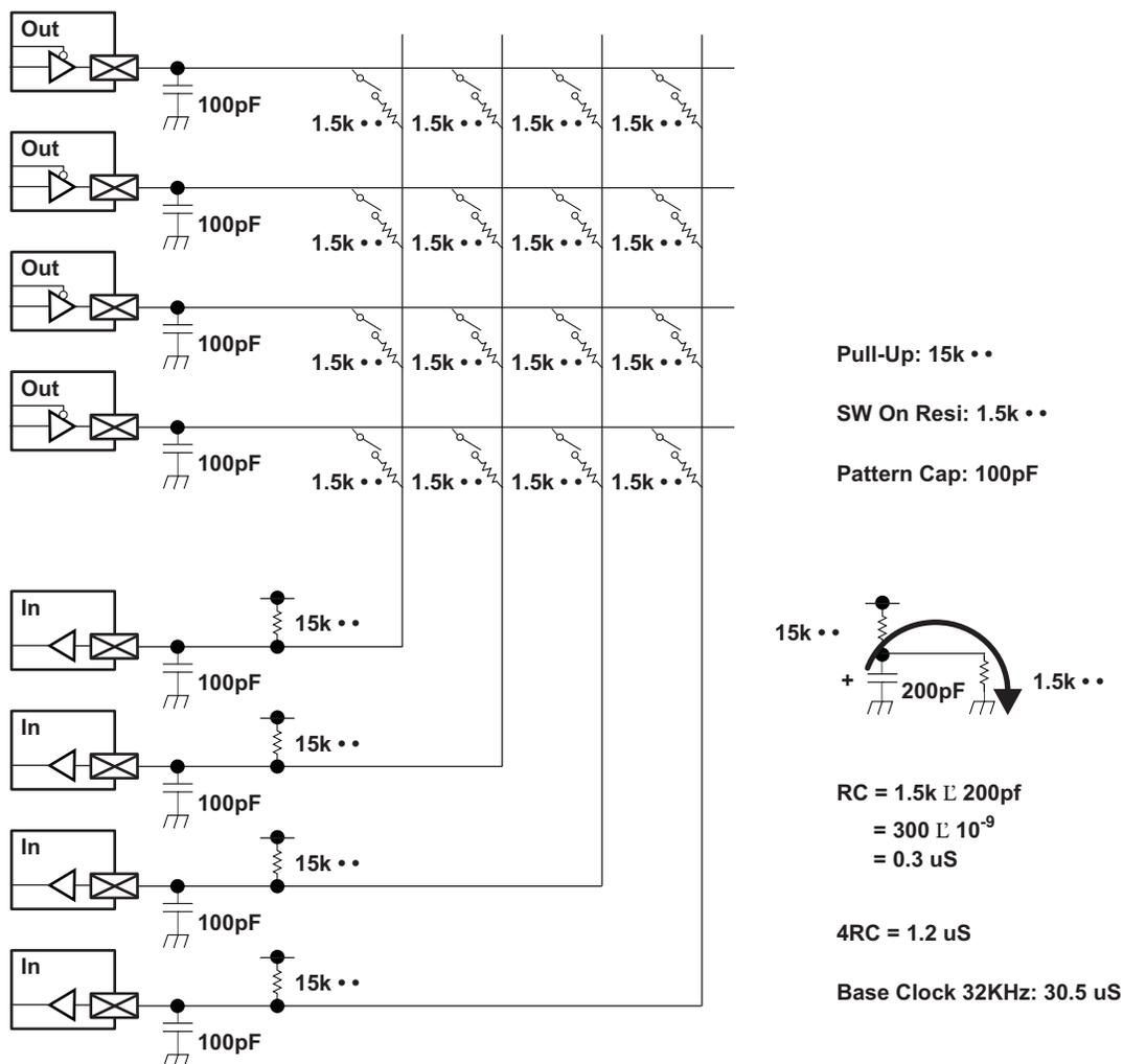
Figure 3. Key Scan External Circuit Diagram (5x3)
