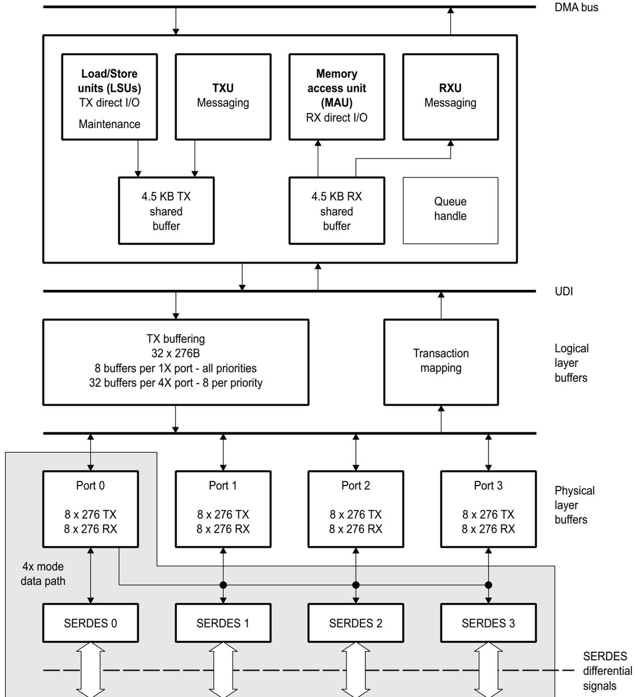
Figure 9. SRIO Component Block Diagram for TMS320TCI6486/87/88/C6472
