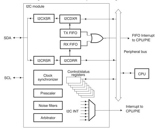
Figure 2. I2C Module Conceptual Block Diagram
