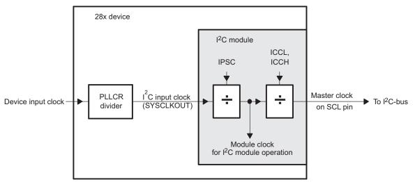
Figure 3. Clocking Diagram for the I2C Module
