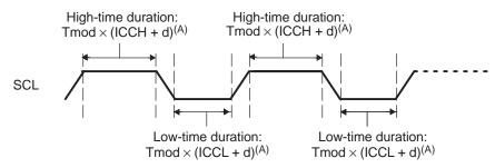
A As described in Section 5.7.1, Tmod is the module clock period, and d is 5, 6, or 7.
