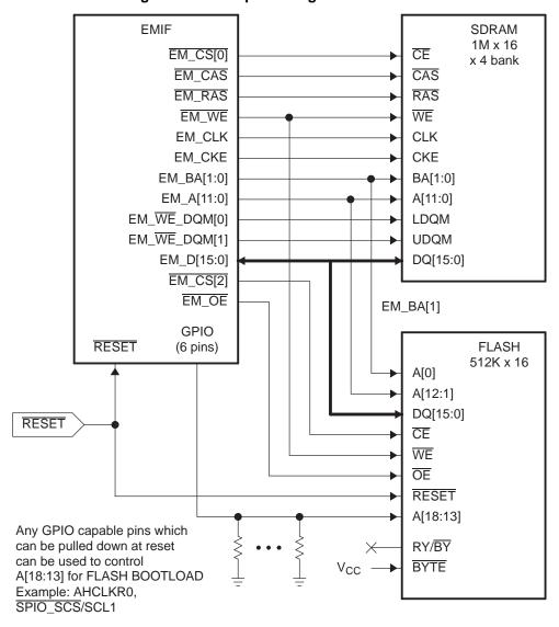
Figure 4-1. Example Configuration Interface
