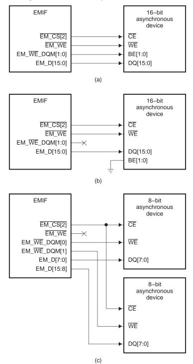
Figure 2-10. Common Asynchronous Interfaces
