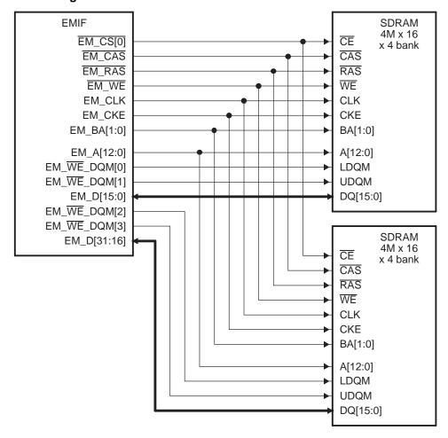
Figure 2-5. EMIF to dual 4M x 16 x 4 bank SDRAM Interface
