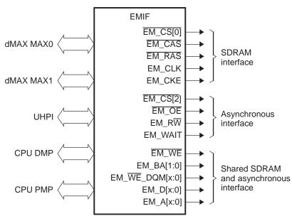
Figure 1-1. EMIF Functional Block Diagram
