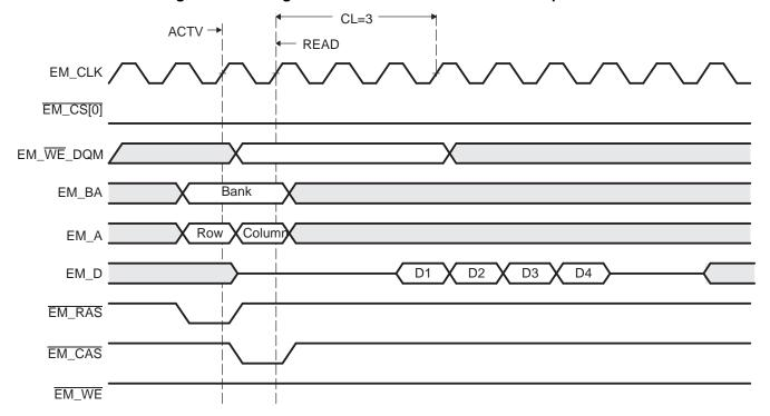
Figure 2-6. Timing Waveform for Basic SDRAM Read Operation
