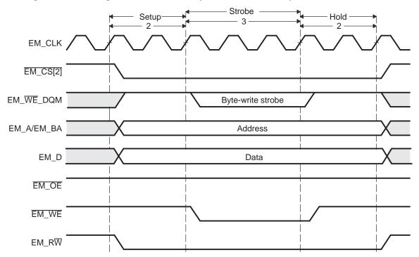
Figure 2-12. Timing Waveform of an Asynchronous Write Cycle in WE Strobe Mode
