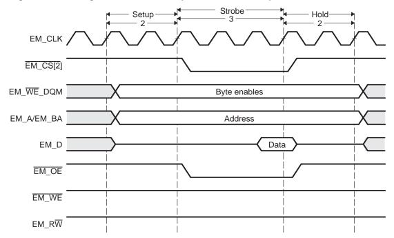
Figure 2-13. Timing Waveform of an Asynchronous Read Cycle in Select Strobe Mode
