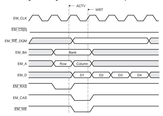
Figure 2-7. Timing Waveform for Basic SDRAM Write Operation
