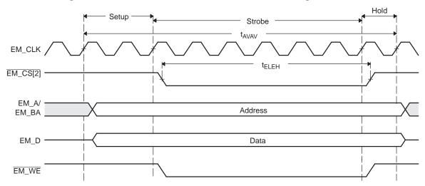
Figure 4-7. LH28F800BJE-PTTL90 to EMIF Write Timing Waveforms
