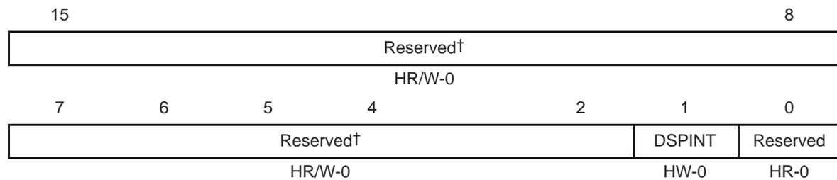
**Legend:** HR/W = Host read/write access; HW = Host write-only access; -n = Value after DSP reset (The DSP cannot access HPIC)
