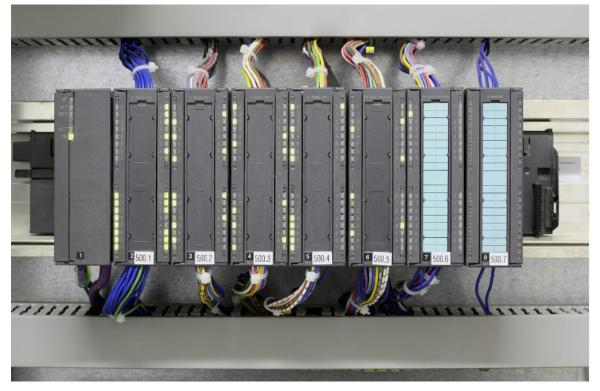
Figure 1. A typical PLC
