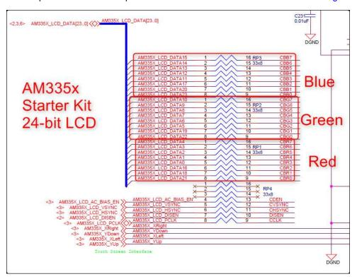
Figure 1. AM335x Starter Kit, 24-Bit LCD
