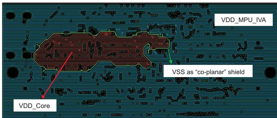
**Figure 8. Example of Co-Planar Shielding of Power Net Using Ground Guard-Band**
