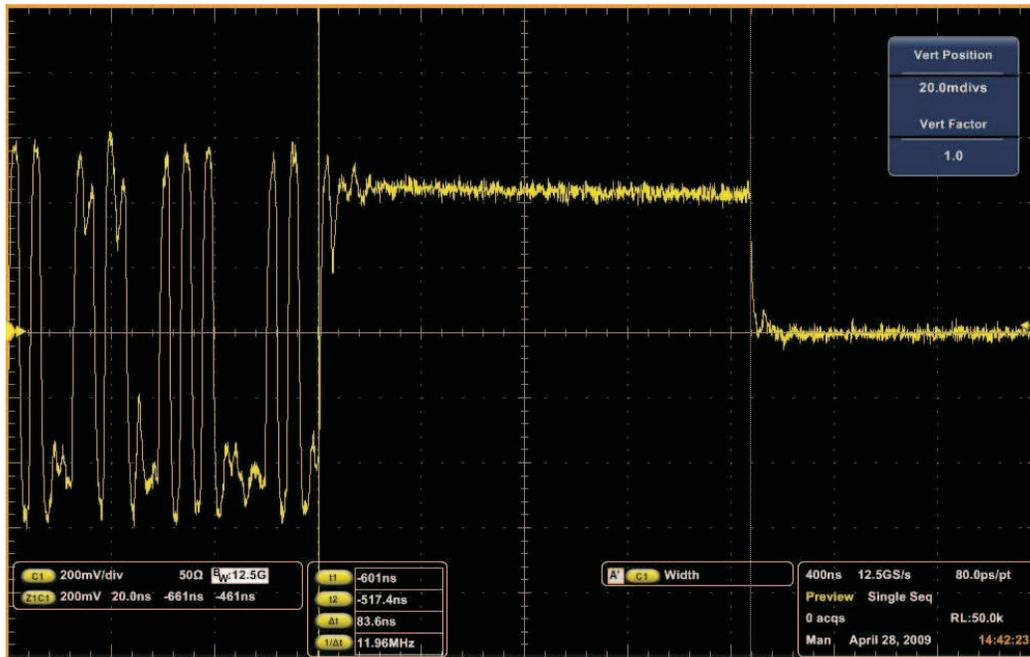
Figure 13. EOP Field of an SOP Packet
