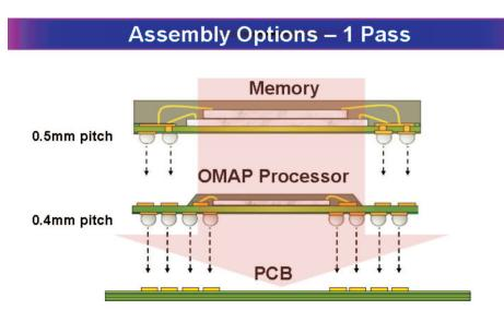
Figure 7. Assembly Options - 1 Pass
