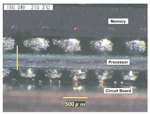
Figure 3. Close-up Of The OMAP35xx Processor And PoP Memory Stack Up
