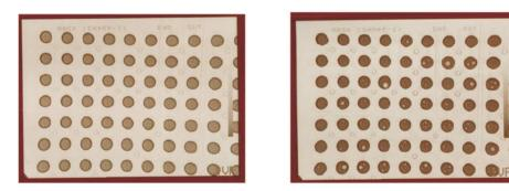
Figure 11. Differences Between Reflow in Nitrogen (left image) and Air (right image) With SnAgCu Solder
