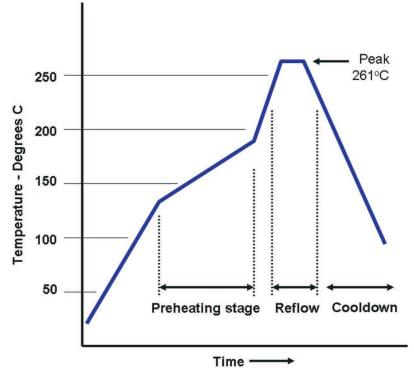
Figure 12. CircuitCo Reflow Profile
