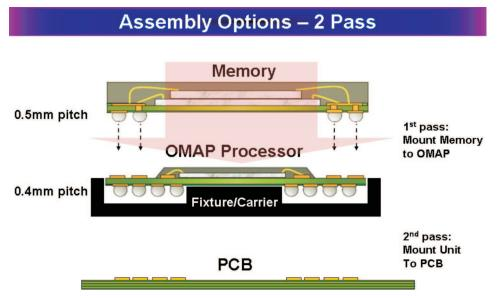
Figure 8. Assembly Options - 2 Pass
