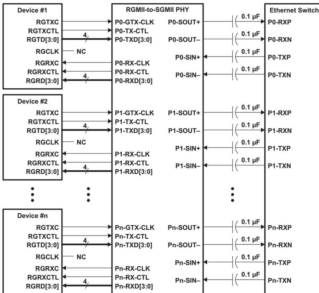
Figure 7. RGMII Switch Connectivity Diagram
