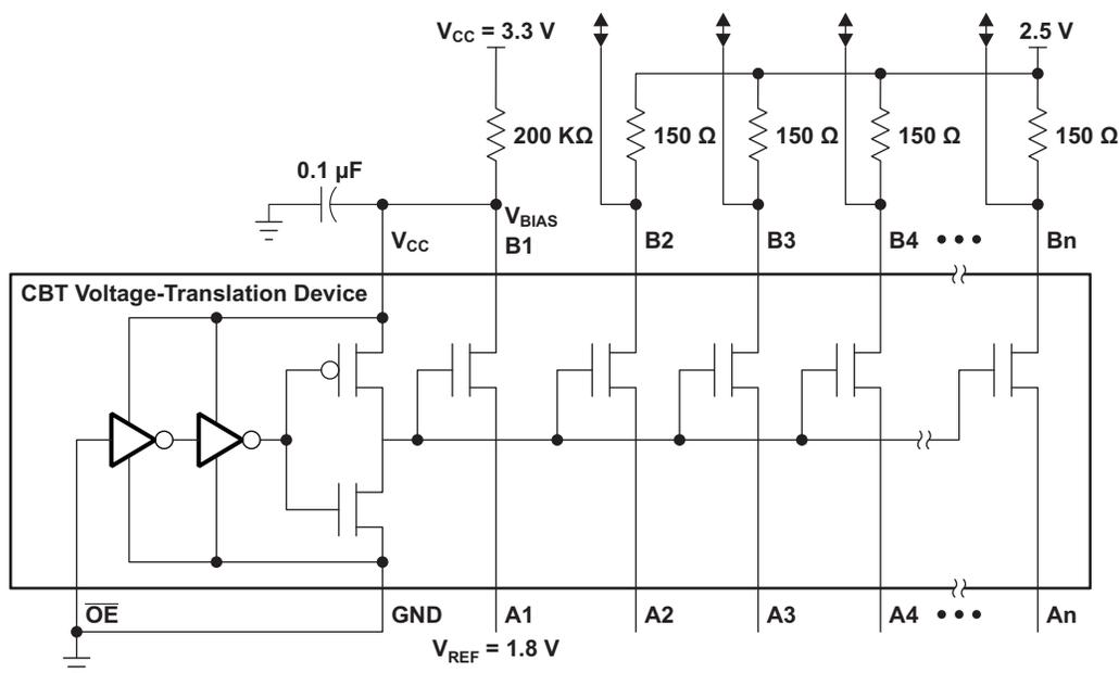
**Figure 13. RGMII Voltage Level Translation Circuit**
