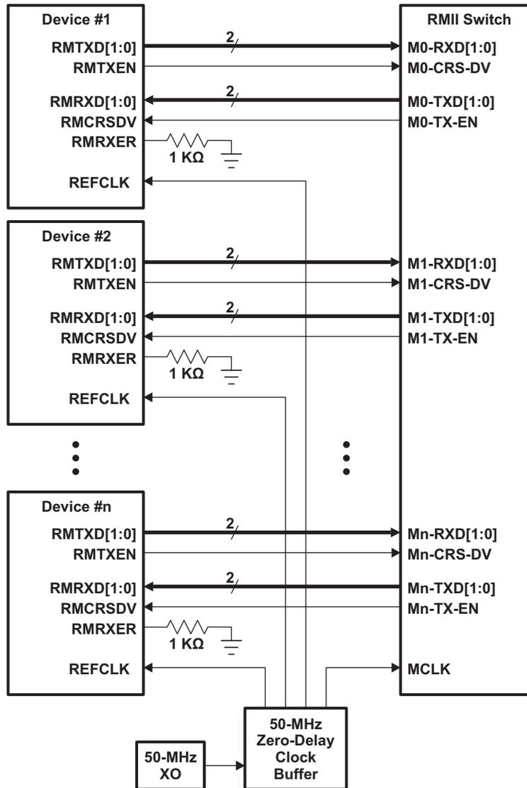
Figure 5. RMI Switch Connectivity Diagram
