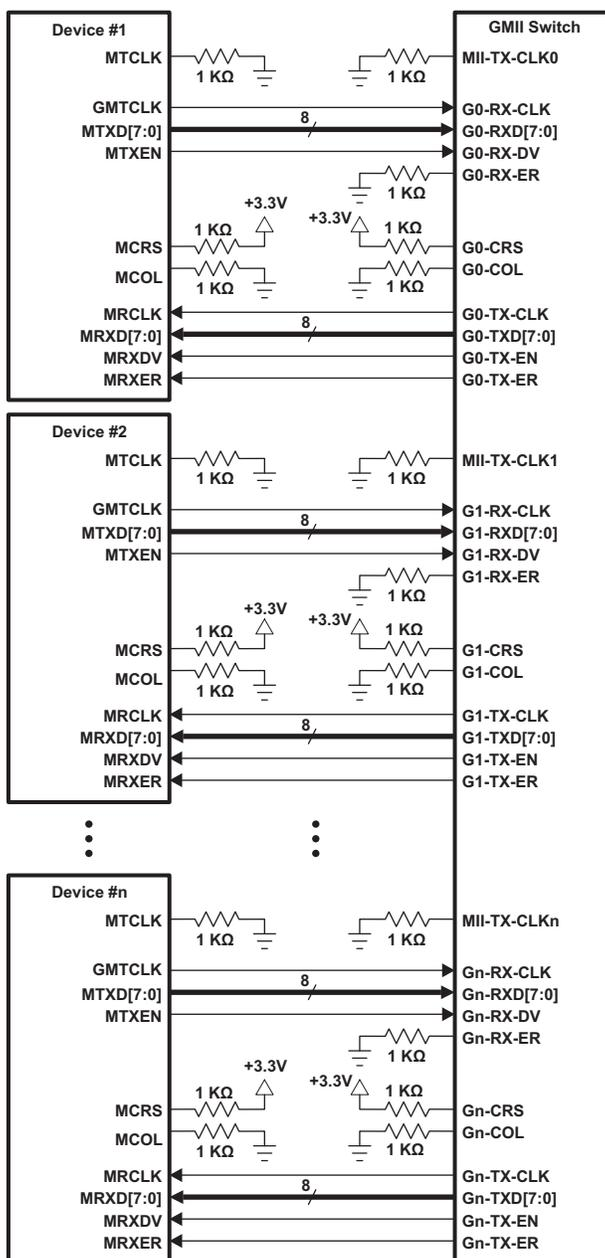
Figure 2. GMII Switch Connectivity Diagram
