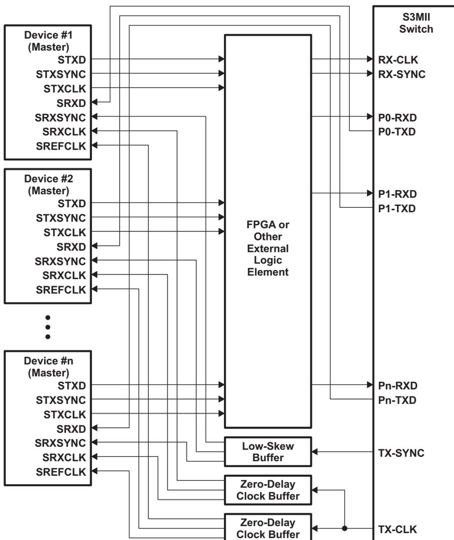
Figure 12. S3MII Multi-Switch Connectivity Diagram
