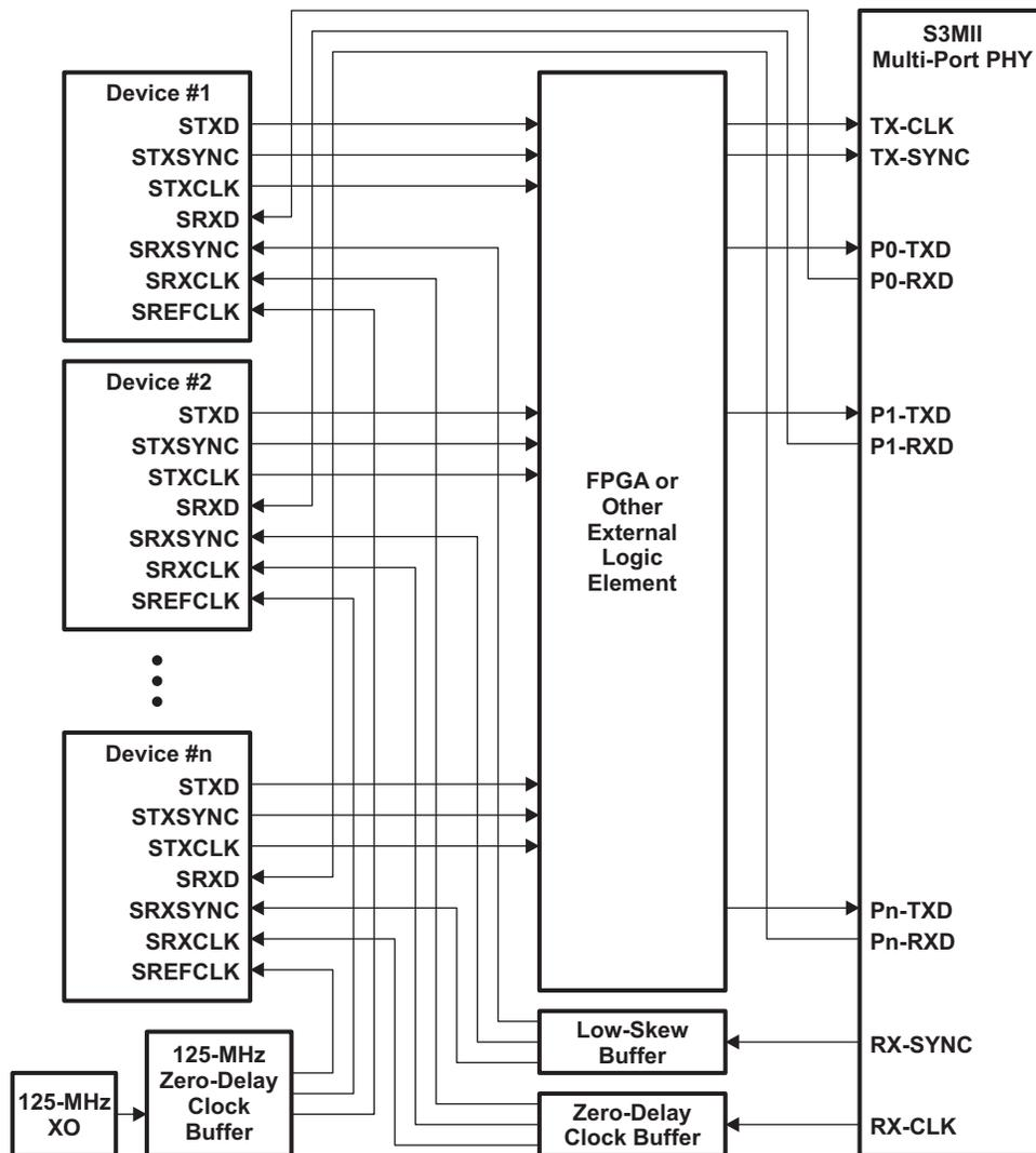
Figure 10. S3MII Multi-Port PHY Connectivity Diagram
