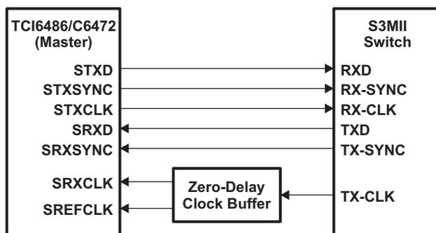
Figure 11. S3MII Switch Connectivity Diagram
