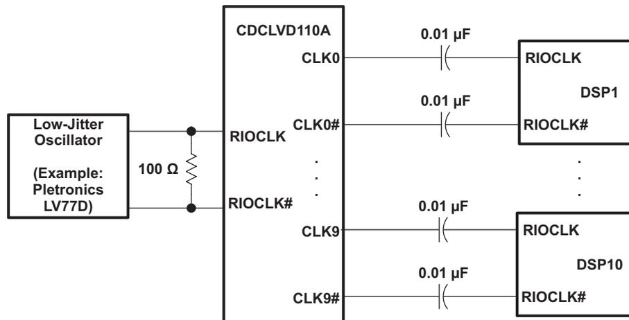
**Figure 7. RIOCLK Multiple Devices LVPECL Clock Solution**
