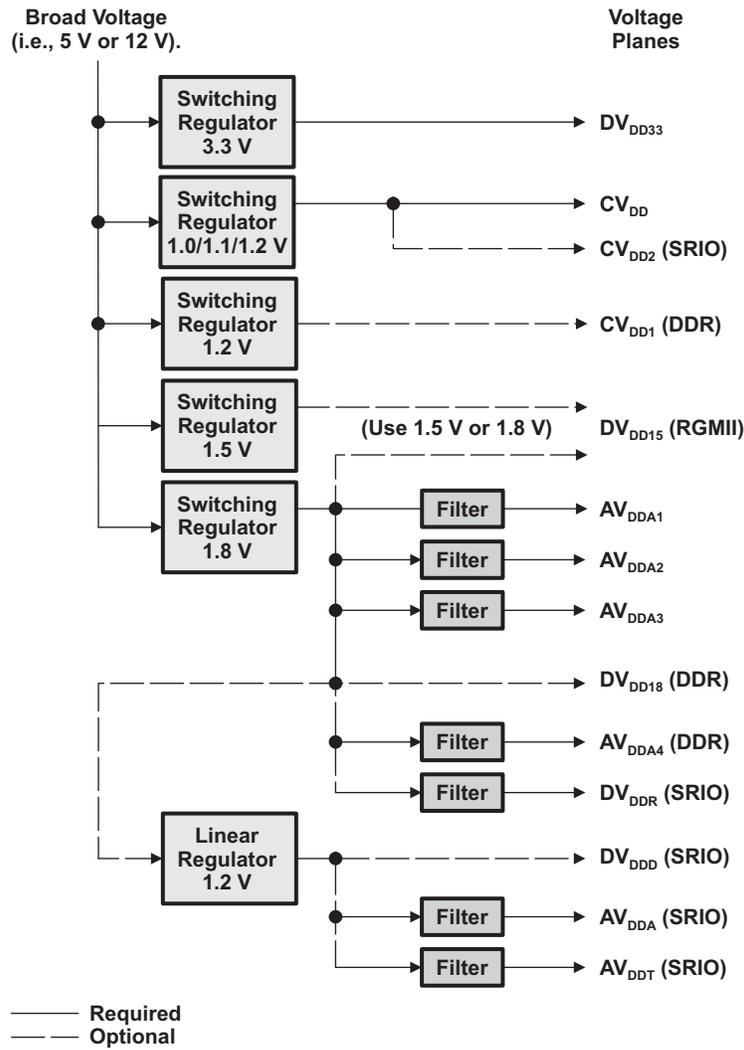
The recommended filter circuit for Figure 8 is given in Figure 9. The filter component shown is a Murata part. If a different part is cross-referenced, the frequency envelope must be considered. This solution has been tested.
