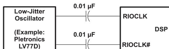
**Figure 5. RIOCLK Single Device LVPECL Clock Solution**
