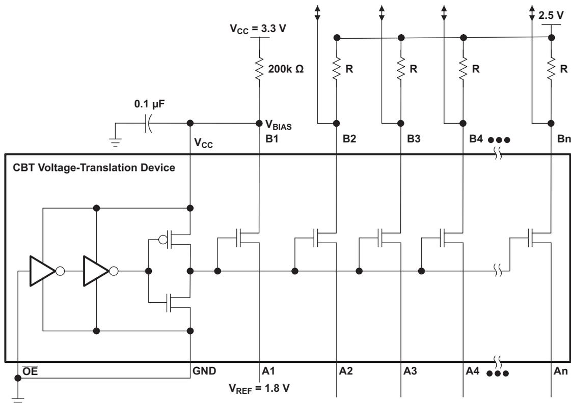
The CBT and TVC families of buffers are excellent in this application. Both are simple FET switches, which offer sub-ns propagation delays. Because each FET switch is independent, the relative delays are matched very closely because process variations affect all switches equally. Unlike LVC MOS buffers, these switches offer no additional current drive, however, since gigabit Ethernet connections are simple point-point connections this is not a concern.
