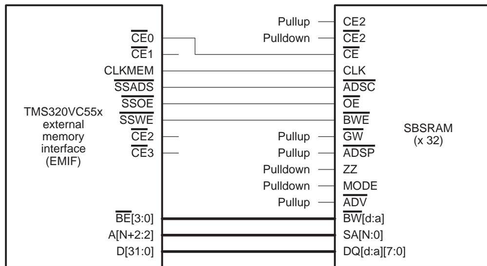
Figure 6. C55x EMIF Interface to Non-parity, Pipeline SBSRAM
