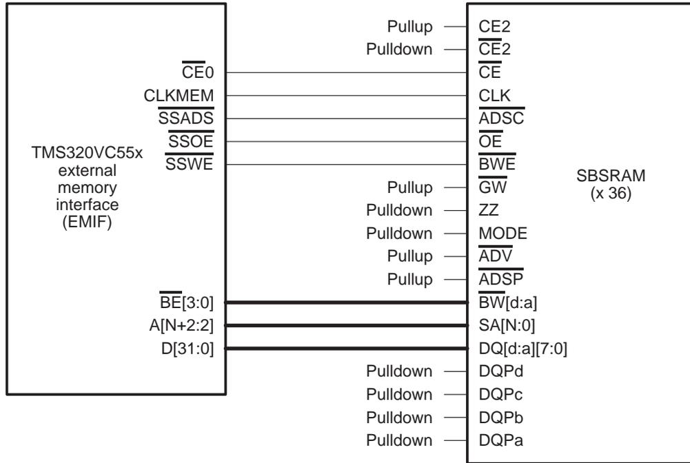
Figure 7. C55x EMIF Interface to Parity (x36), Pipeline SBSRAM
