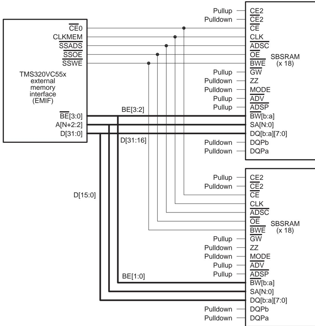
Figure 8. C55x EMIF Interface to 2 Parity (x18), Pipeline SBSRAMs
