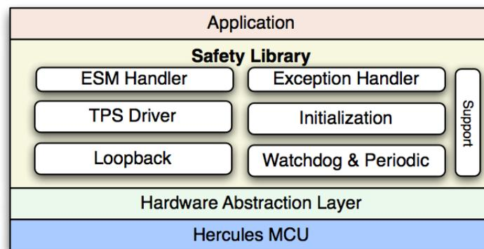
**Figure 1. Software Stack With SafeTI Diagnostic Library**
