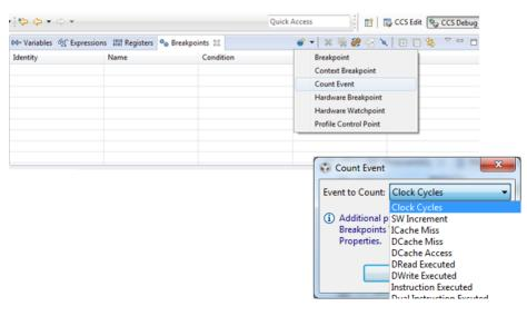
Figure 4. PMU Profiling in CCS
