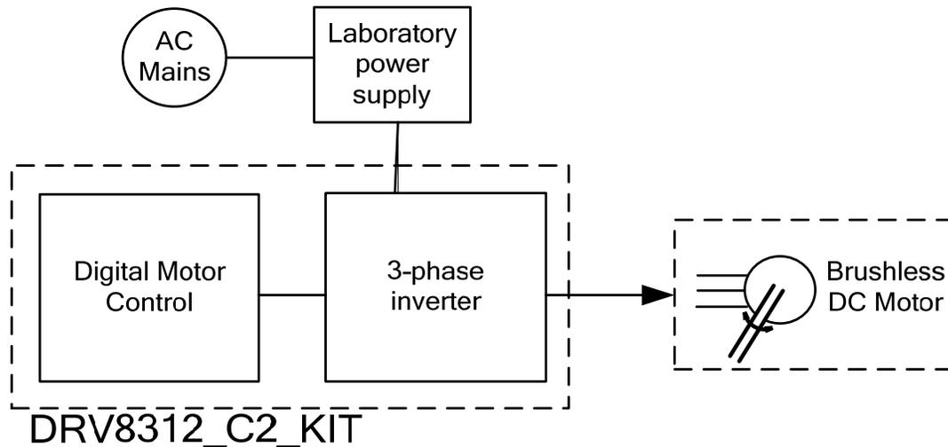
Figure 3. Typical Motor Drive System Block Diagram
