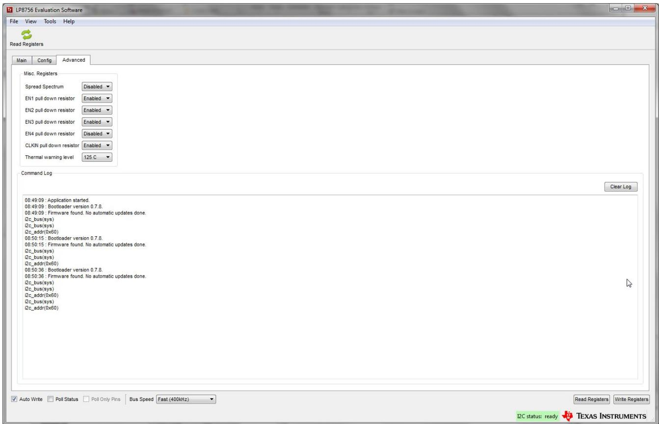
**Figure 17. Advanced Tab of LP8756 GUI**
