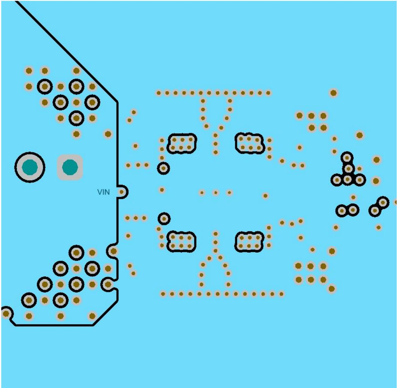
VIN supply is routed in this layer between the ground planes to reduce radiated emissions. VIN and GND vias are placed in hatched pattern to avoid large gaps in these planes.
