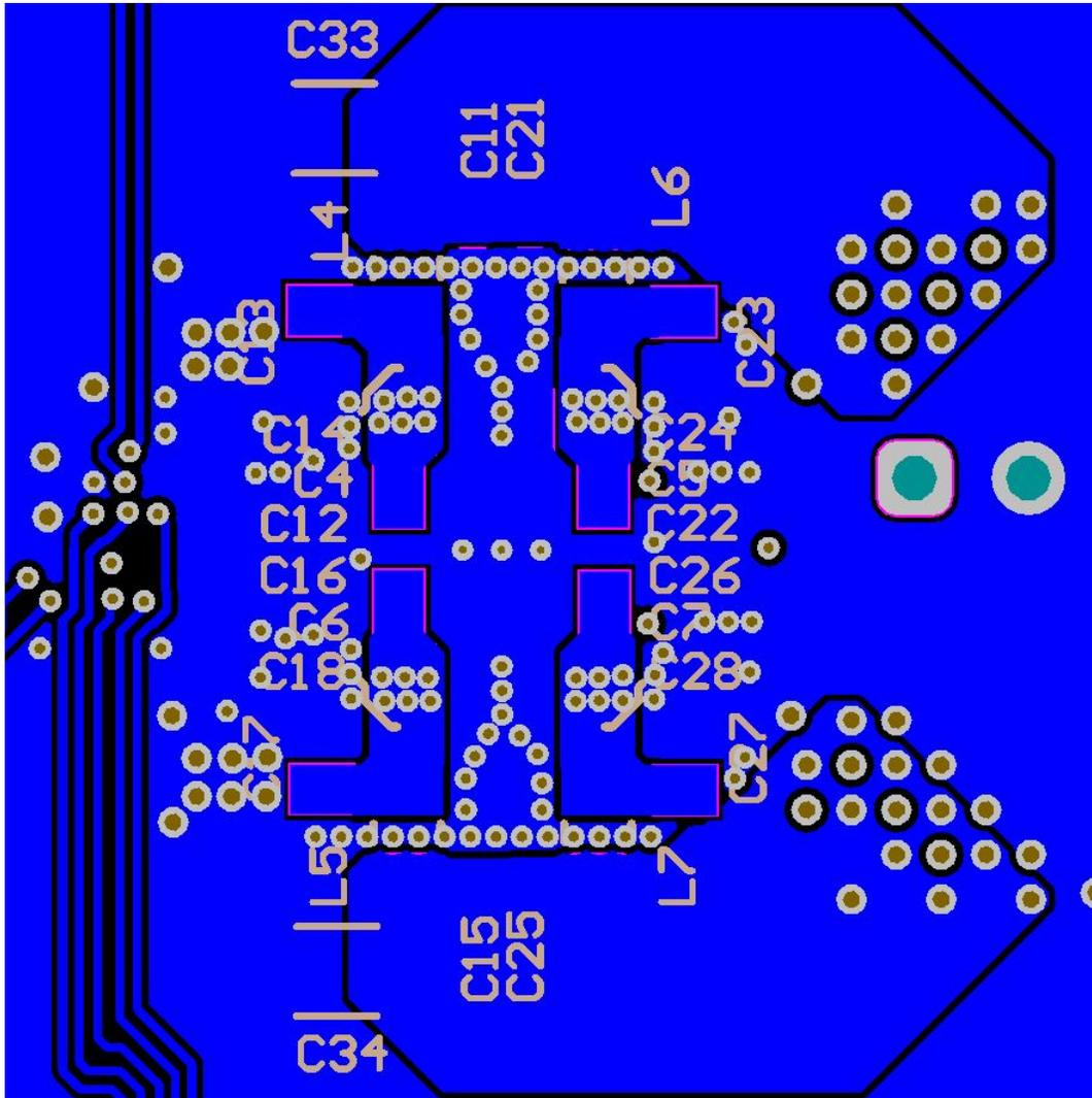
Input capacitors and filters are placed under the LP8756xQ1 into bottom layer. This allows closer placement of the inductors and input components reducing SW and VIN net areas and improving EMI.
