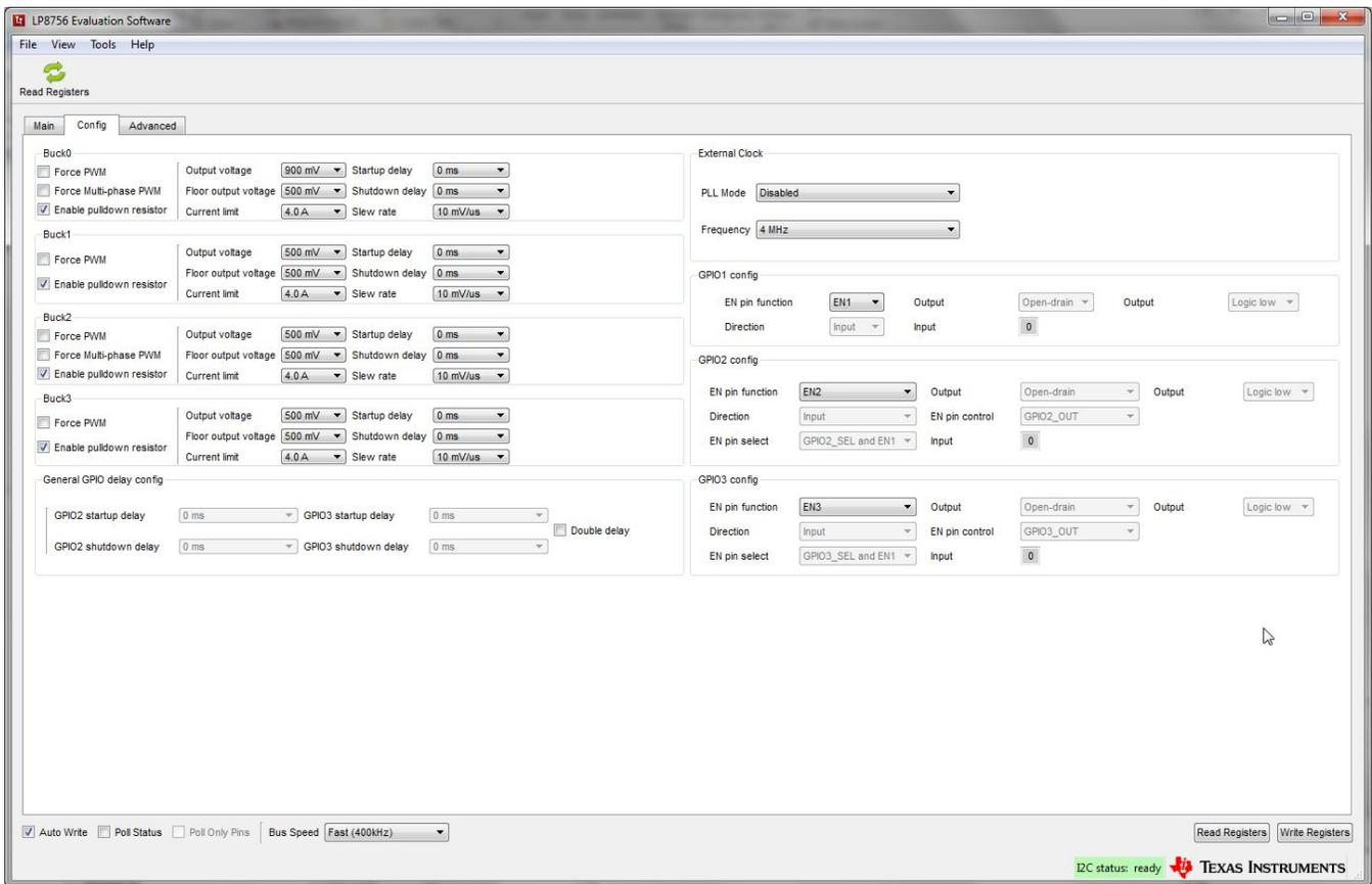
Figure 9. Config Tab of the LP8756 GUI
