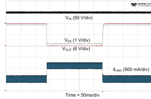
$V_{IN} = 48\text{ V}$        $F_{SW} = 300\text{kHz}$        $V_{OUT} = 12\text{ V}$
