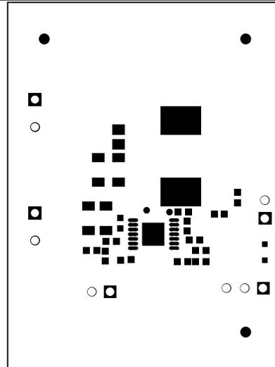
Figure 24. EVM Top Solder Mask with LM5161
