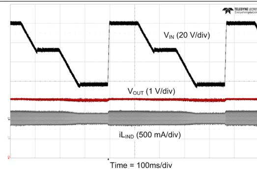
$F_{SW} = 300\text{kHz}$        $V_{OUT} = 12\text{ V}$        $I_{Load} = 500\text{ mA}$
