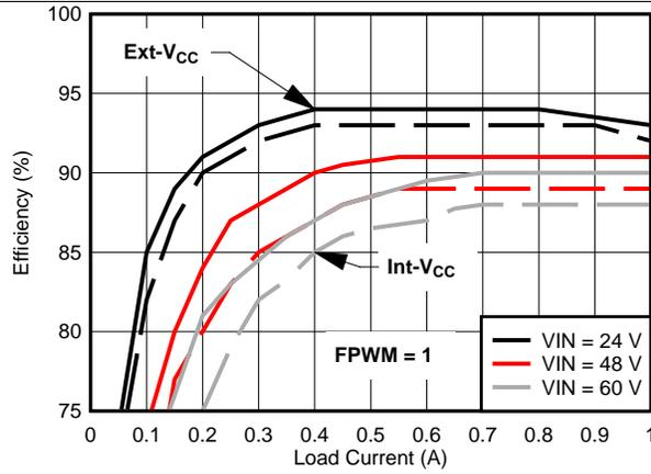
$V_{OUT} = 12\text{ V}$        $FPWM = 1$        $F_{SW} = 300\text{ kHz}$
