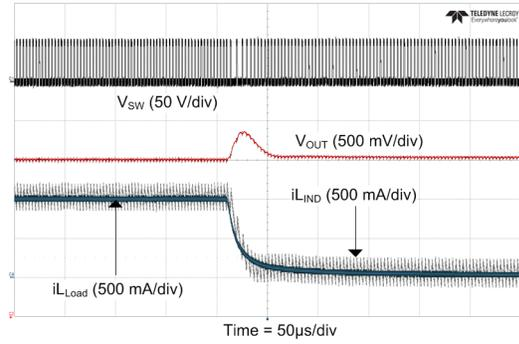
$V_{IN} = 48\text{ V}$        $FPWM = 1$        $F_{SW} = 300\text{kHz}$        $V_{OUT} = 12\text{ V}$
