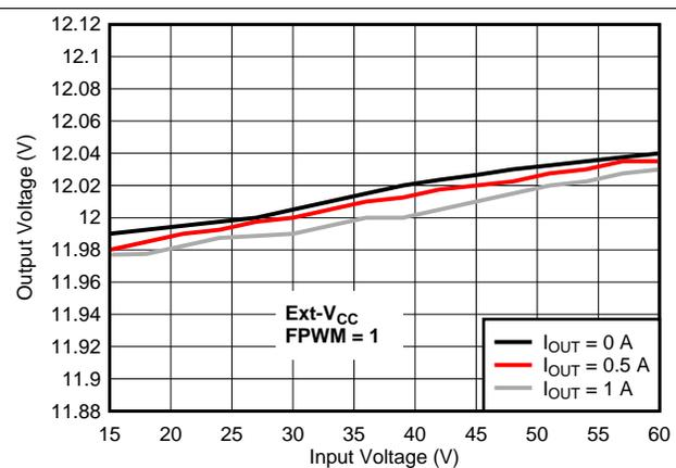
$V_{\text{OUT}} - V_{\text{CC}}$  diode connected      FPWM = 1       $F_{\text{SW}} = 300\text{kHz}$
