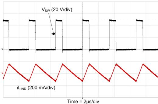
Figure 8. Steady State at  $V_{IN} = 48\text{ V}$  and  $FPWM = 1$  (no load)
