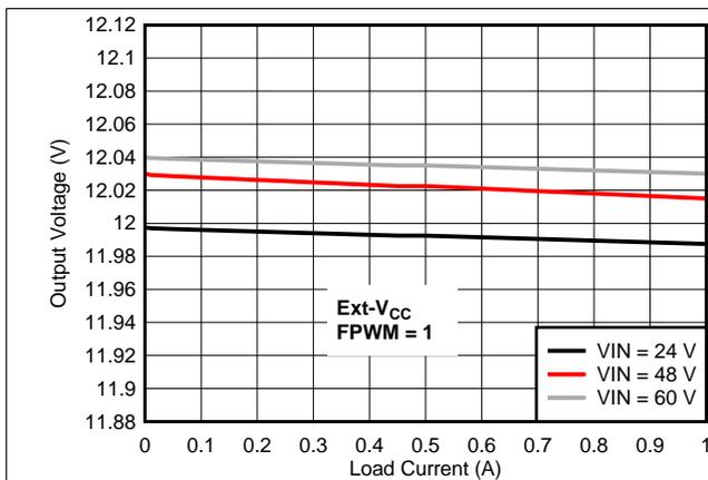
$V_{\text{OUT}} - V_{\text{CC}}$  diode connected      FPWM = 1       $F_{\text{SW}} = 300\text{kHz}$
