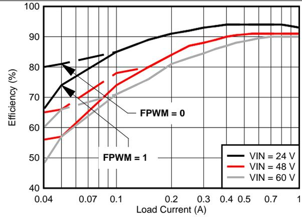
$V_{OUT} - V_{CC}$  diode connected       $F_{SW} = 300\text{ kHz}$        $V_{OUT} = 12\text{ V}$
