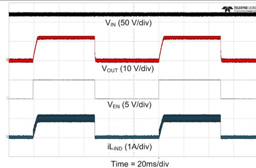
$V_{IN} = 48\text{ V}$        $F_{SW} = 300\text{ kHz}$        $FPWM = 1$        $V_{OUT} - V_{CC}$  diode connected
