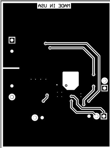
Figure 23. EVM Bottom Copper View with LM5161
