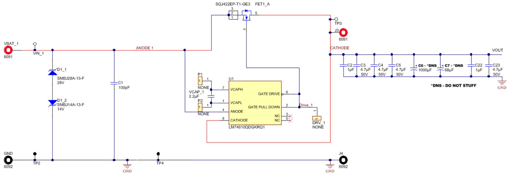
Figure 9. LM74610-SQEVM Schematic
