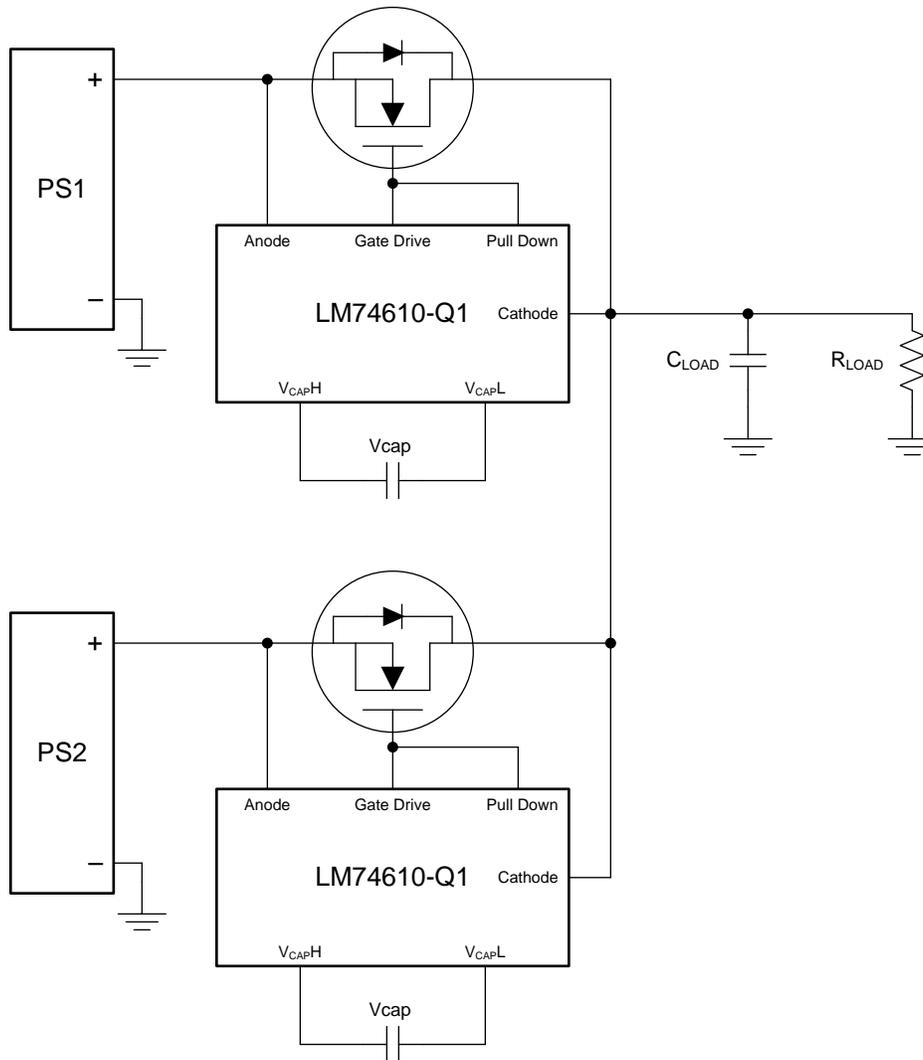
**Figure 1. LM74610-Q1 Typical OR-ing Application Circuit**
