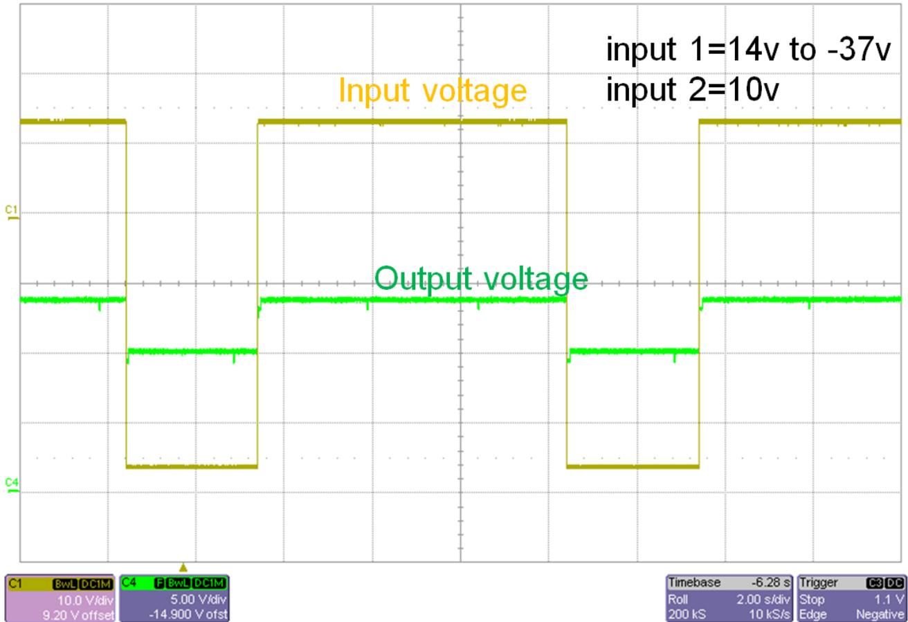
Figure 8. ORing Application for One DC Input and One Dynamic Pulse
