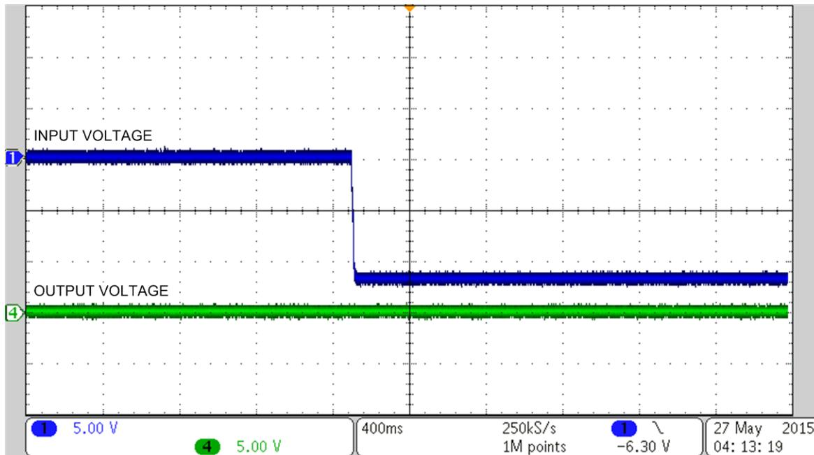
**Figure 4. Response to Start Up Reverse Polarity**
