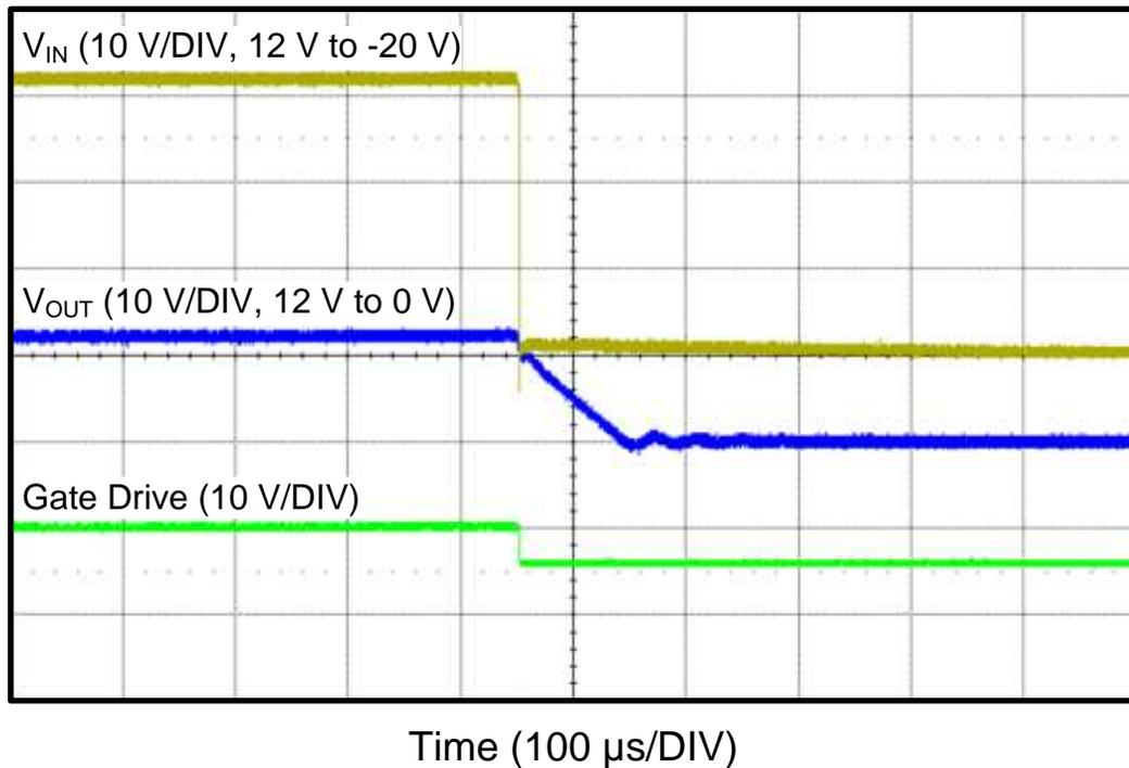
**Figure 3. Response to Reverse Polarity 12V to -20V**
