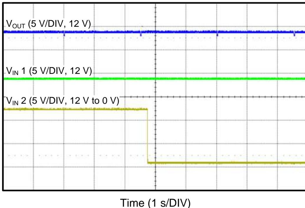
**Figure 9. LM74610-Q1 OR-ing Waveform**
