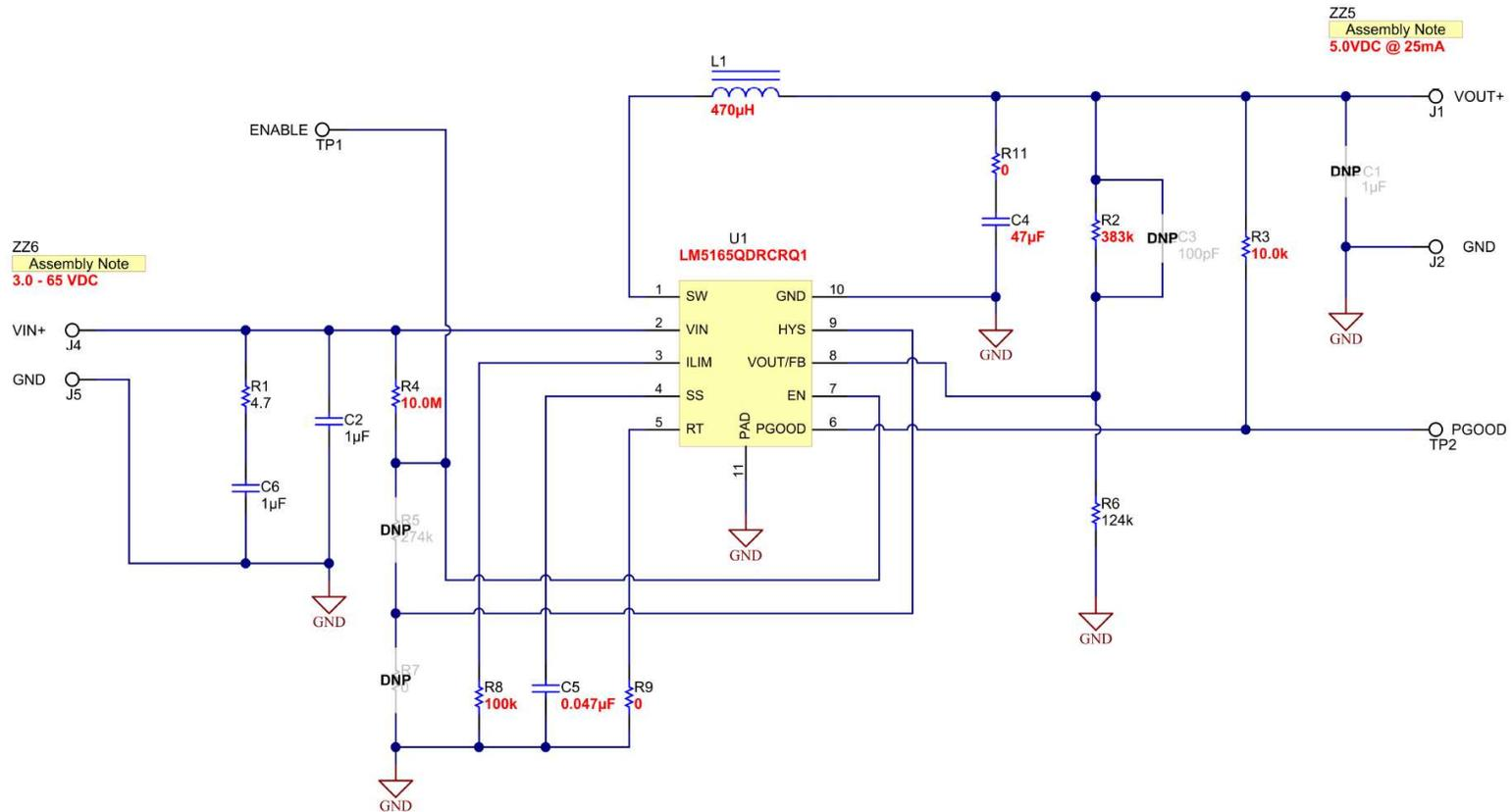
Figure 13. 5V, 25mA PFM Schematic (Adjustable Output Version)
