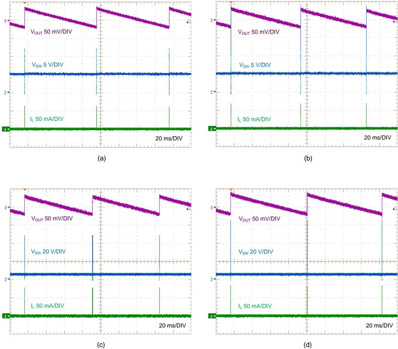
Figure 5. SW Node,  $V_{OUT}$  and  $I_L$  Waveforms at  $I_{OUT} = 0\text{ mA}$ : (a)  $V_{IN} = 12\text{ V}$ , (b)  $V_{IN} = 24\text{ V}$ , (c)  $V_{IN} = 36\text{ V}$ , (d)  $V_{IN} = 65\text{ V}$
