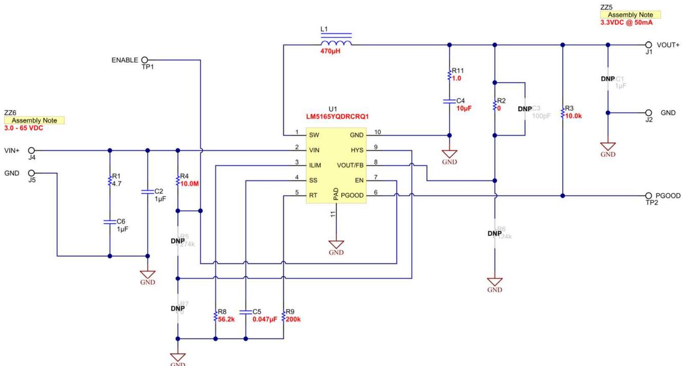
Figure 21. COT, 3.3V, 50mA Schematic (Fixed 3.3V Output Version)
