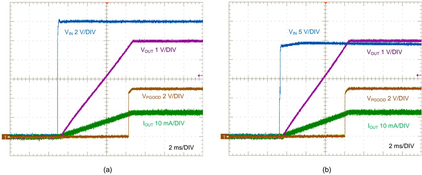
Figure 8. Startup at  $I_{OUT} = 12.5 \text{ mA}$ : (a)  $V_{IN} = 12 \text{ V}$ , (b)  $V_{IN} = 24 \text{ V}$
