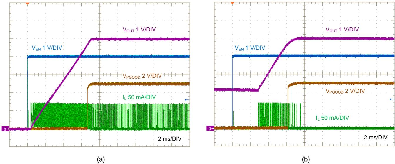
Figure 9. Enable ON at  $V_{IN} = 24 \text{ V}$ : (a)  $I_{OUT} = 12.5 \text{ mA}$ , (b) No Load, 2-V Output Pre-bias
