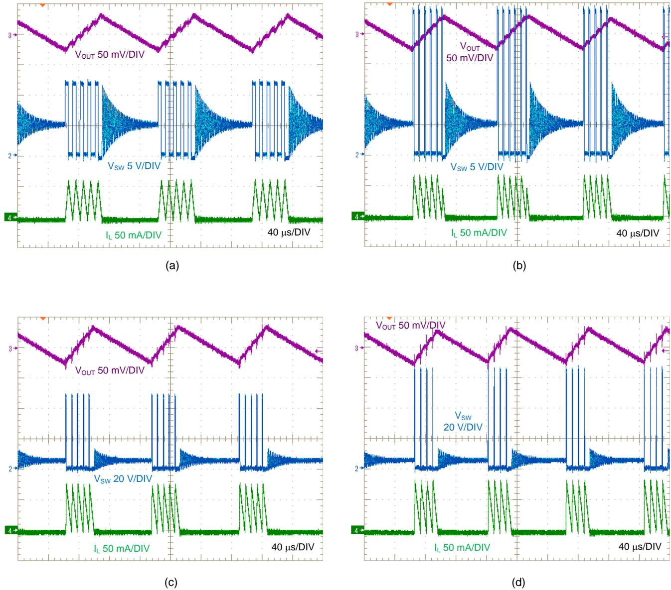
Figure 6. SW Node,  $V_{OUT}$  and  $I_L$  Waveforms at  $I_{OUT} = 12.5$  mA: (a)  $V_{IN} = 12$  V, (b)  $V_{IN} = 24$  V, (c)  $V_{IN} = 36$  V, (d)  $V_{IN} = 65$  V
