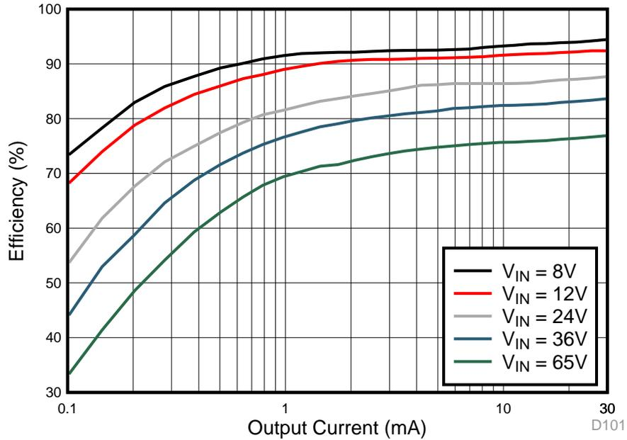
Figure 4. PFM Converter Efficiency, V<sub>OUT</sub> = 5 V
