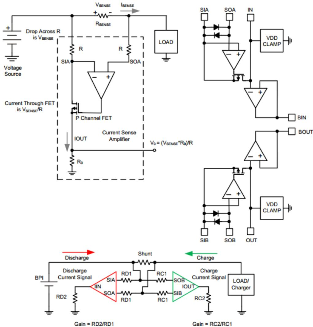
Figure 2. Current Sense Amplifier Connections
