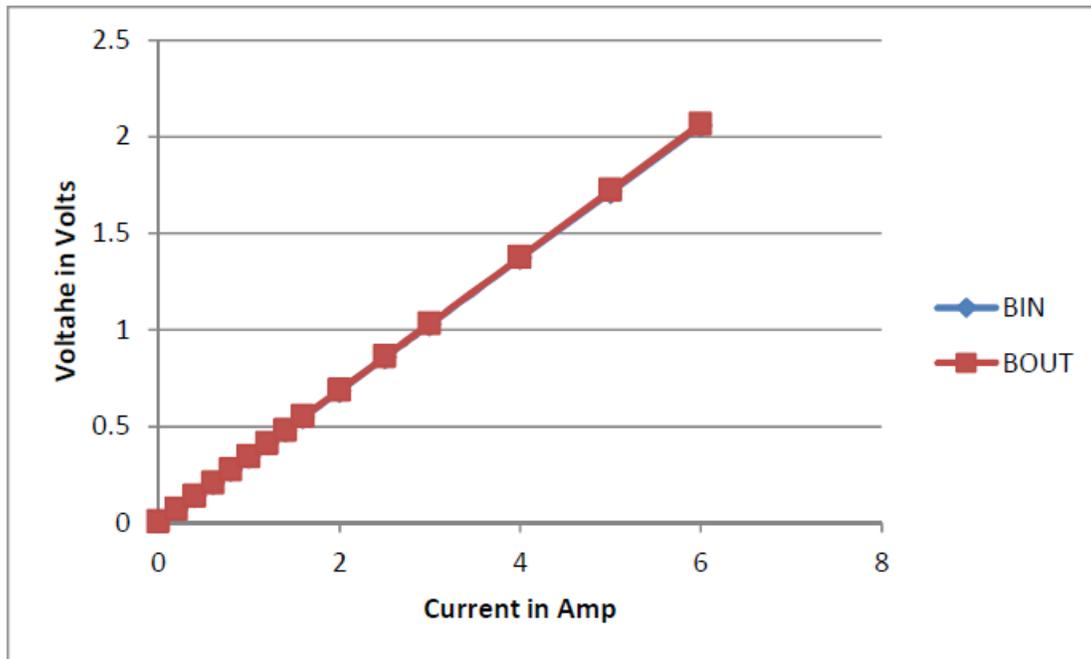
Note: Measurement was taken at 12-V Input at J1 and with Electronic Load at J2 at room temperature (21°C)
