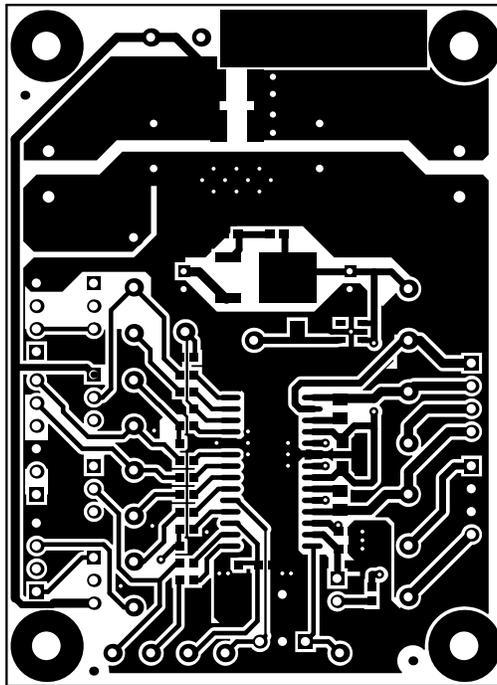
**Figure 5. Top Routing Layer**
