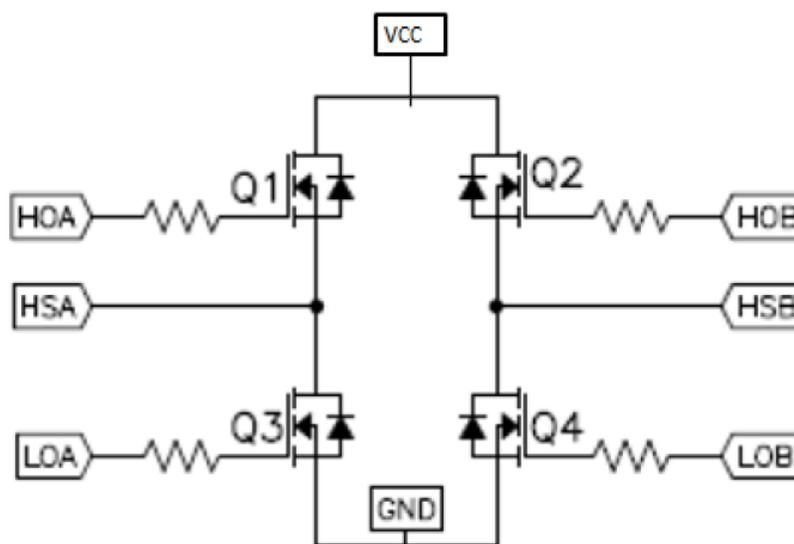
Figure 1. Typical Full Bridge Application - Gate Signals
