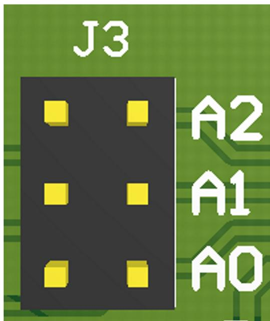
Figure 2-5. I<sup>2</sup>C Slave Select Jumper
