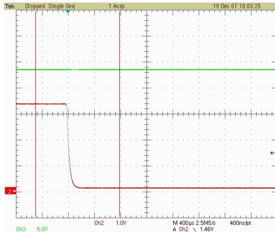
FIGURE 21, Typical protection after short circuit of the 3.3V
