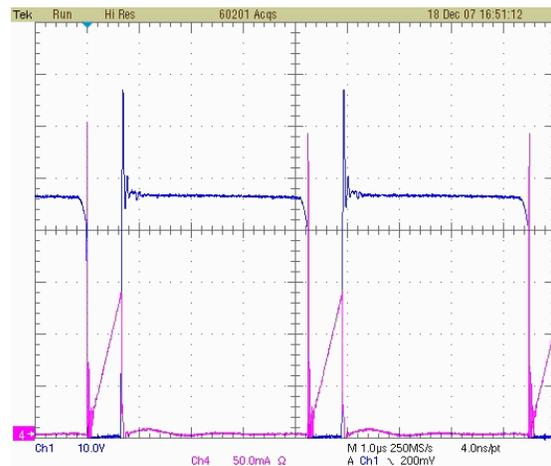
FIGURE 13. One complete cycle:  $V_{IN\ max}$  with  $I_{OUT\ max}$
