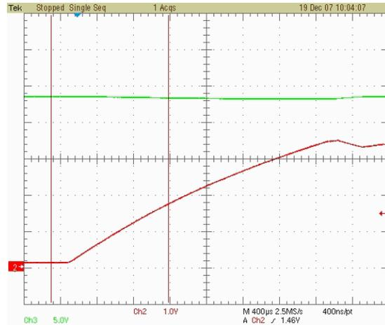
FIGURE 23, Start up phase after that the short circuit is removed
