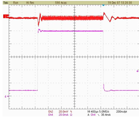
**FIGURE 16, Load Transient**
