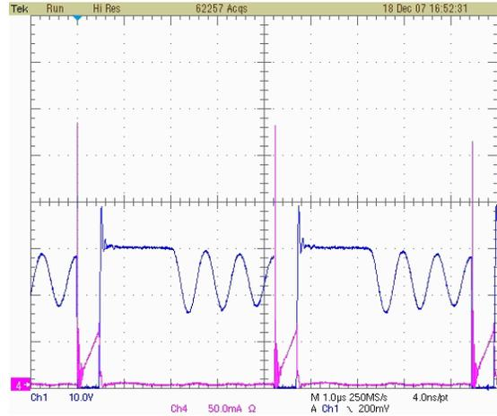
**FIGURE 107. Output regulation: Minimum load at 24V<sub>in DC</sub>**
