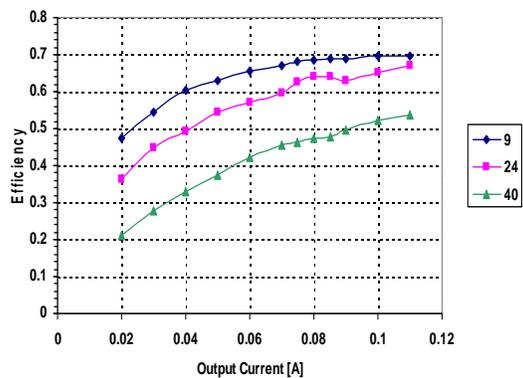
**FIGURE 156, Efficiency of the DC/DC part: no input filter and no bridge**
