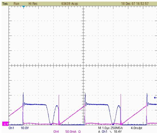
**FIGURE 16. One complete cycle:  $V_{IN\ min}$  with  $I_{OUT\ min}$**
