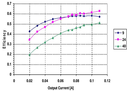
**FIGURE 14, Efficiency of the complete board without the input filter at  $V_{in}=9V, 24V, 40V$**
