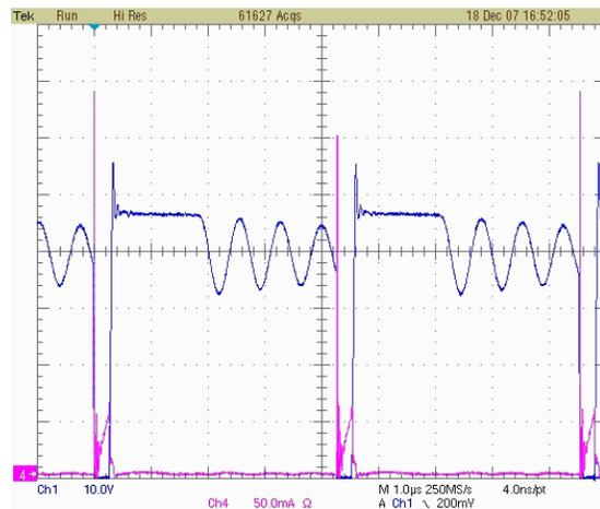
FIGURE 14. One complete cycle:  $V_{IN\ max}$  with  $I_{OUT\ min}$
