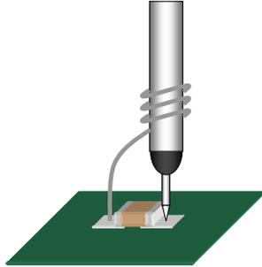
FIGURE 6. Short Probe Connection
