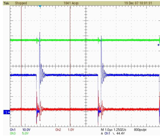
FIGURE 22, Typical protection after short circuit of the 3.3V
