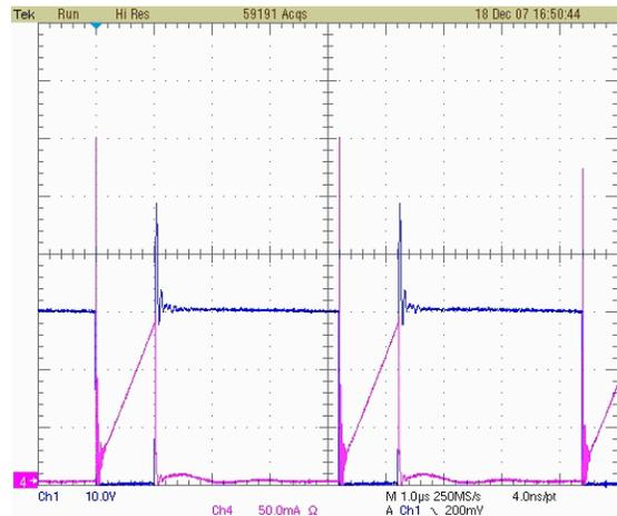
**FIGURE 118. Output regulation: Maximum load at 24V<sub>in DC</sub>**
