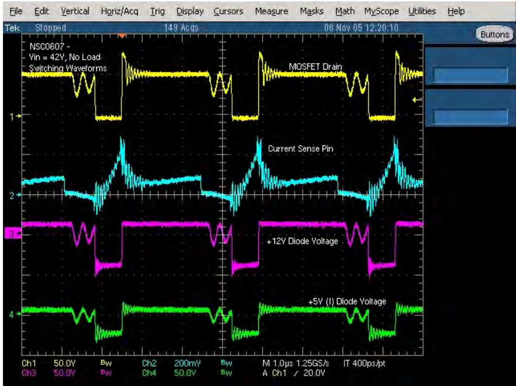
FIGURE 14. Switching waveforms, Vin=42V
