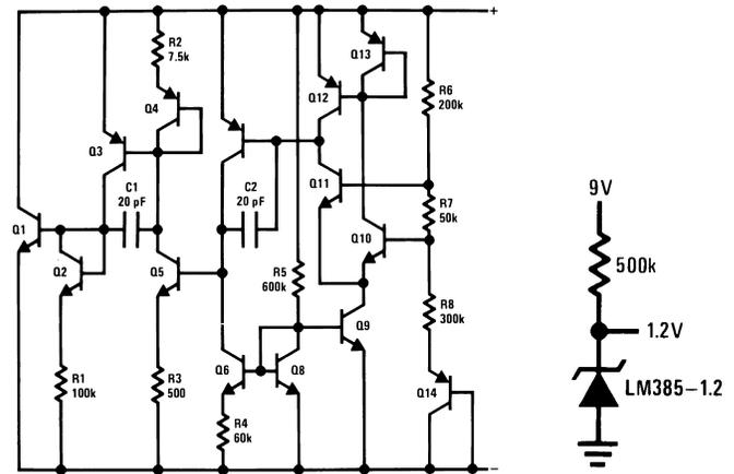
Fig. 1 LM185H-1.2RLQV simplified schematic and application diagram.
