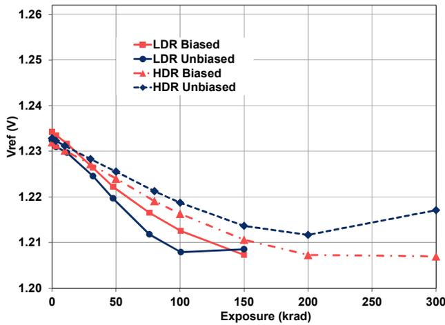
Fig. 2 Reference voltage at 10  $\mu$ A operating current.
