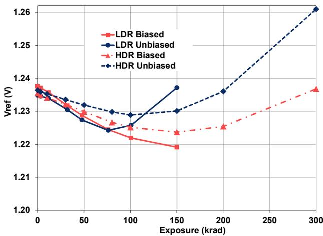
Fig. 4 Reference voltage at 20 mA operating current.
