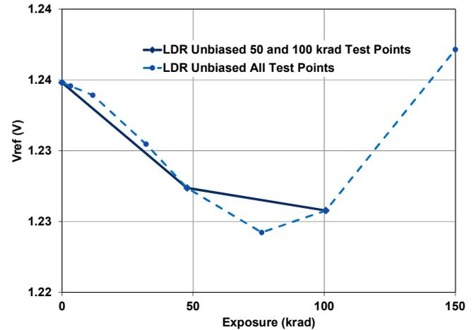
Fig. 6 Reference voltage at 20 mA operating current, LDR with units unbiased during irradiation. The dashed line shows the curve for all test points measured. The solid line represents what might be assumed about the TID drift in test points were only take at the rated value and half the rated value.
