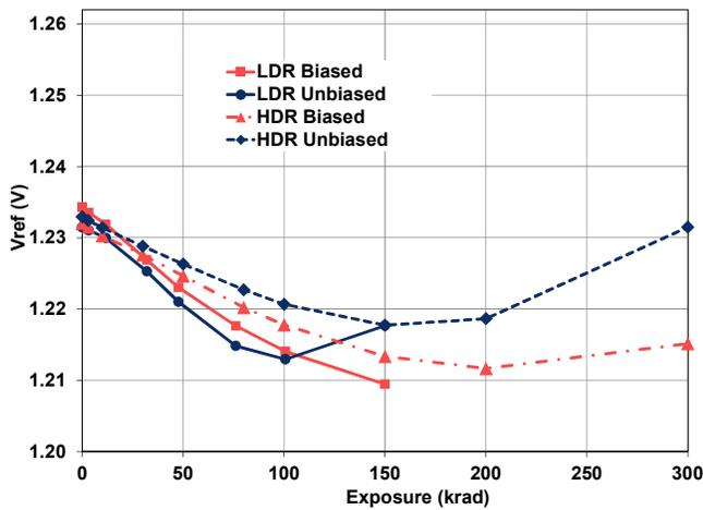
Fig. 3 Reference voltage at 1 mA operating current.
