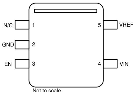
**Figure 4-1. DBV Package 5-Pin SOT-23 Top View**
