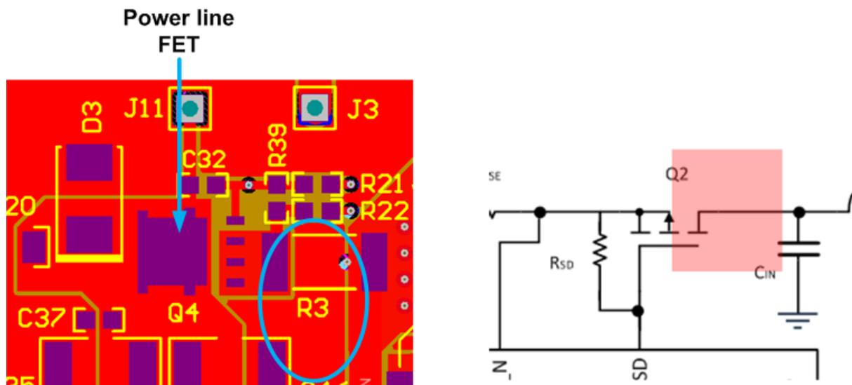
**Figure 17. Recommended PCB Pad for Power-Line FET**
