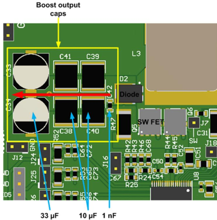
Figure 19. Recommended Placement of Boost Output Capacitors
