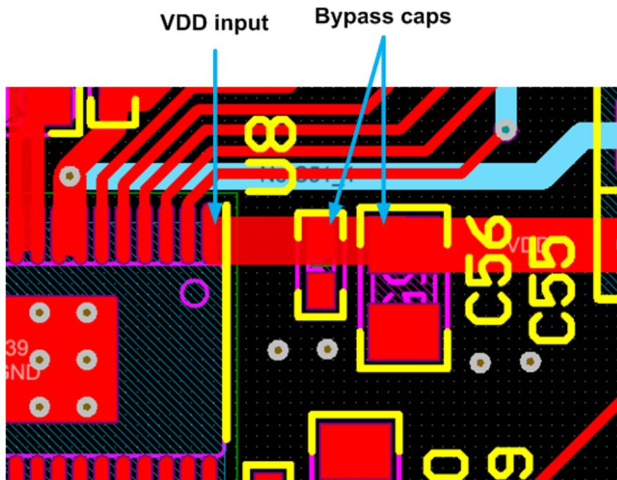
Figure 14. Bypass Capacitors of Logic Power Input
