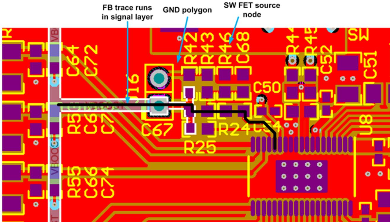
Figure 15. Trace for Boost Feedback
