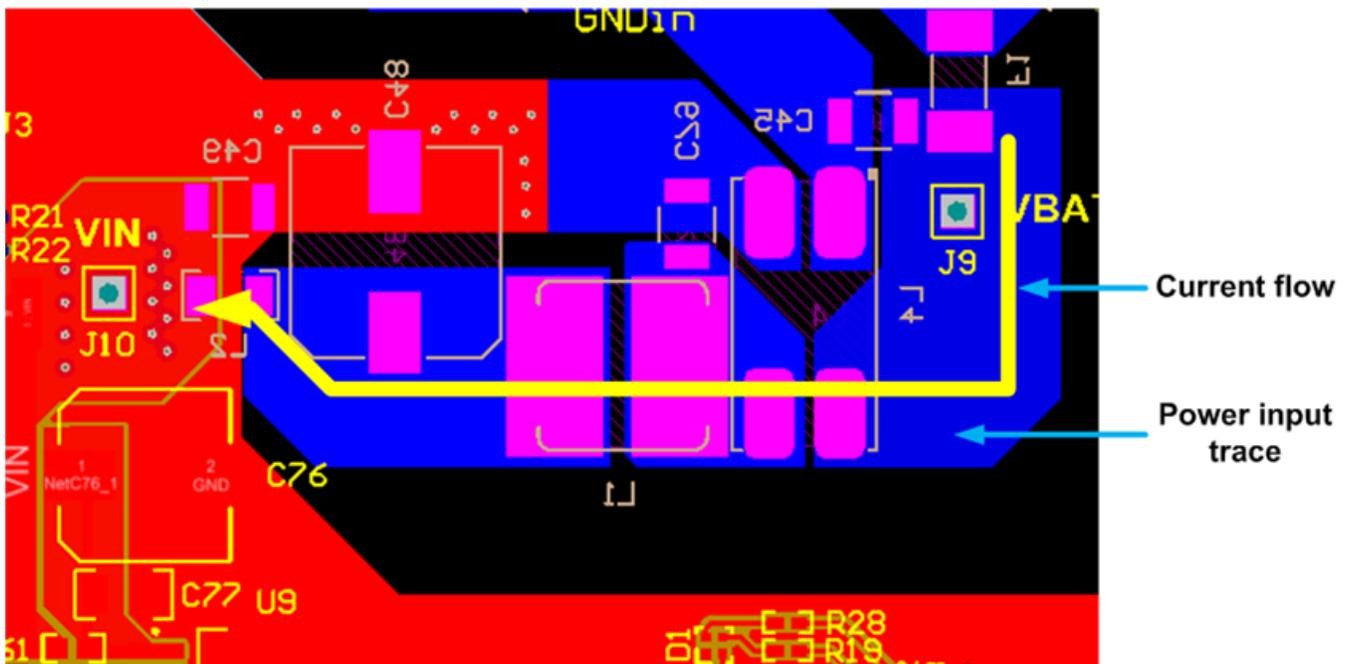
**Figure 18. Boost Input Power (V<sub>IN</sub>) Trace**
