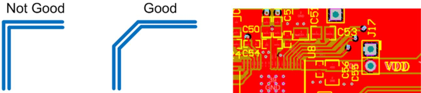
Figure 20. Recommended Trace Routing of Digital Signals
