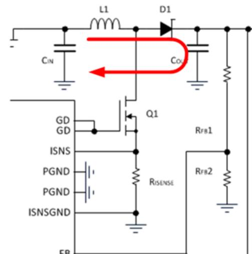
Figure 7 shows main current flows and component placements. Power ground of input, switch, and boost output are all centered and each component has enough vias to connect to ground plane with shortest path.
