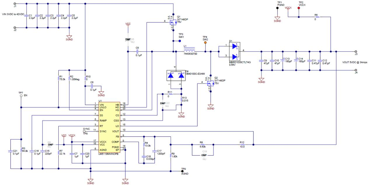
**Figure 4. Test Board Schematic: Reference Design PMP 10681**
