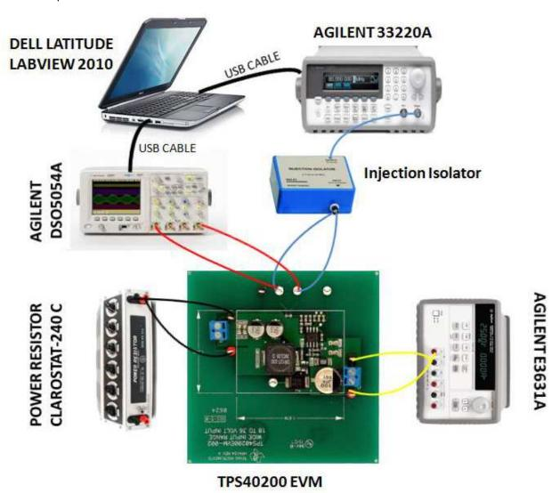
Figure 8. Concept Validation (System Setup)
