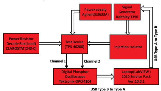
Figure 1. System Level Block Diagram
