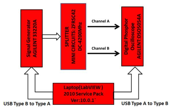
Figure 6. Oscilloscope Characterization (Test Setup)
