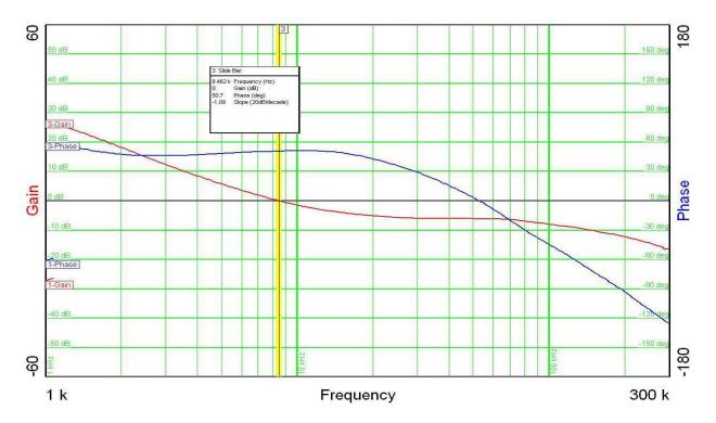
Figure 17. Loop Gain Response Given in User Guide
