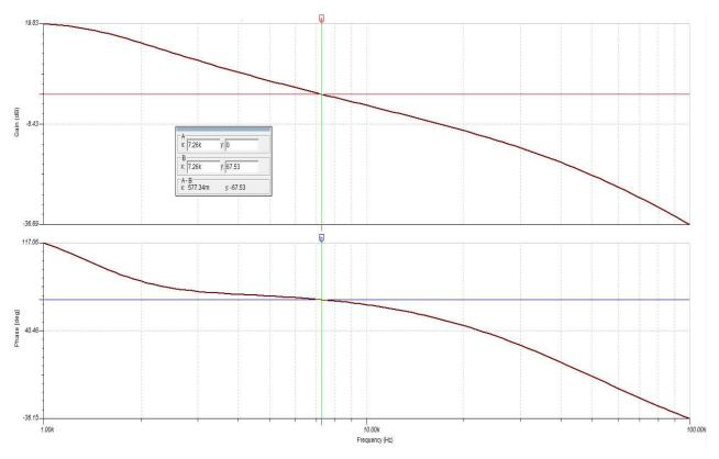
Figure 13. TINA-TI Loop Gain Plot
