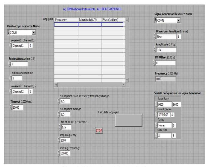
Figure 5. GUI Front Panel Using LabVIEW™
