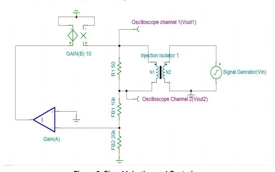
Figure 2. Signal Injection and Capturing
