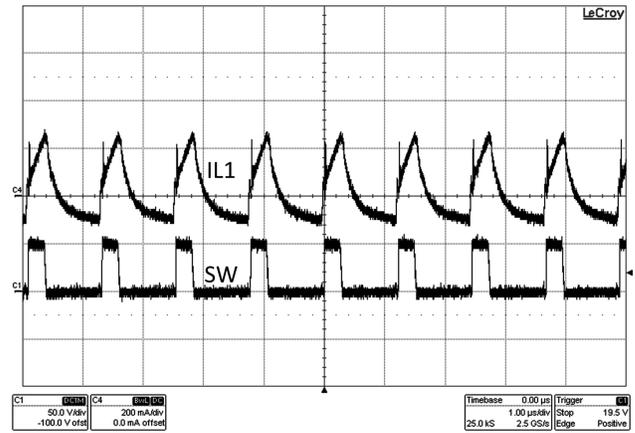
Figure 4. Steady State Waveform (VIN = 48V, IOUT1 = 0mA, IOUT2 = 100mA)
