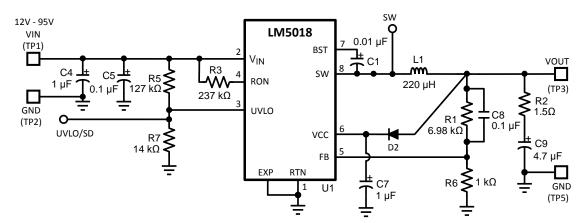
Figure 2. Complete Evaluation Board Schematic for LM5018 Based Buck Converter
