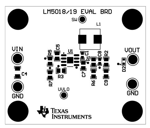
Figure 1. Evaluation Board (Top View)
