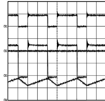
**Figure 6.**  $V_{IN} = 18\text{ V}$ ,  $I_{OUT} = 3\text{ A}$  Illustrating Buck Operation
